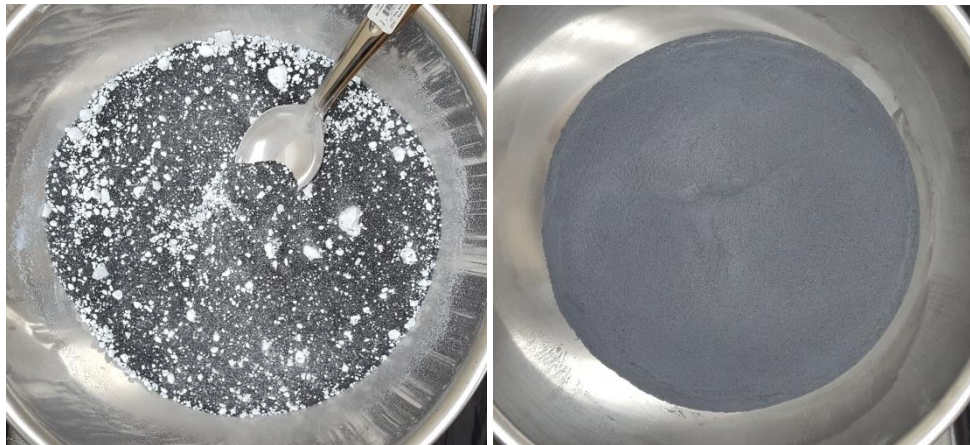
Figure 6 - Carbon and binder mixture before and after blending, left and right, respectively.
