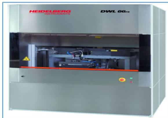
Figure 3.21. Heidelberg 66FS Laser Pattern Generator
