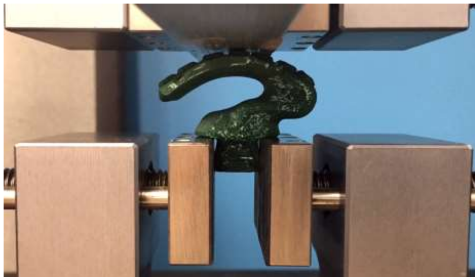
FIGURE 65- Mechanical Stress Testing Of The Prosthetic Foot.
