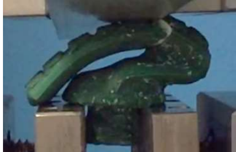
FIGURE 68- Ultimate Failure Of The Prosthetic Device.
