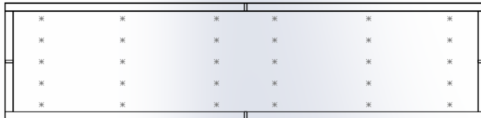
Figure 3-15 Measurement locations for Log-Tchebycheff method
