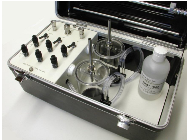
Figure 3-23 Helium Bubble Generator Model 5 (Sage Action, 2016)
