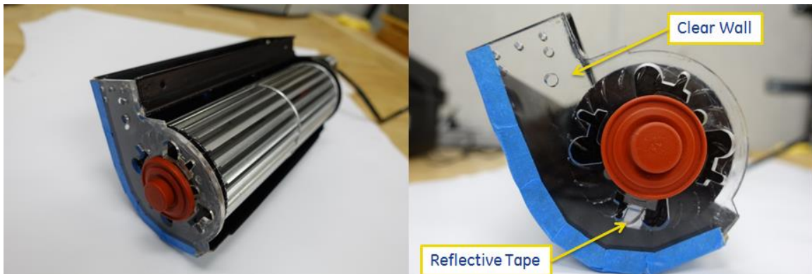
Figure 3-18 Cross-flow fan used in the experiment
