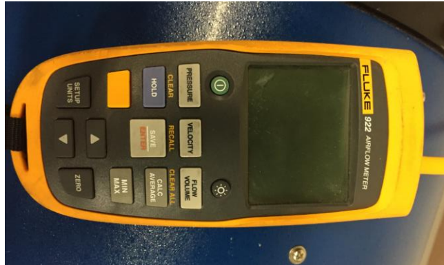
Figure 3-16 Fluke 922 digital manometer
