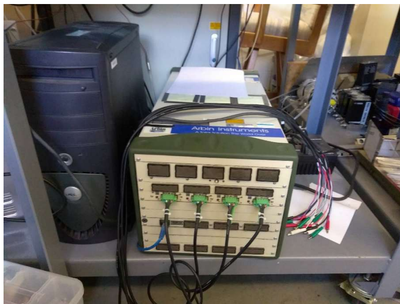
Figure 15. Arbin BT2043™ instrument used for cell cycling.
