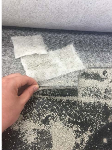
Figure 4-3. The base GCL, Bentomat 200R
