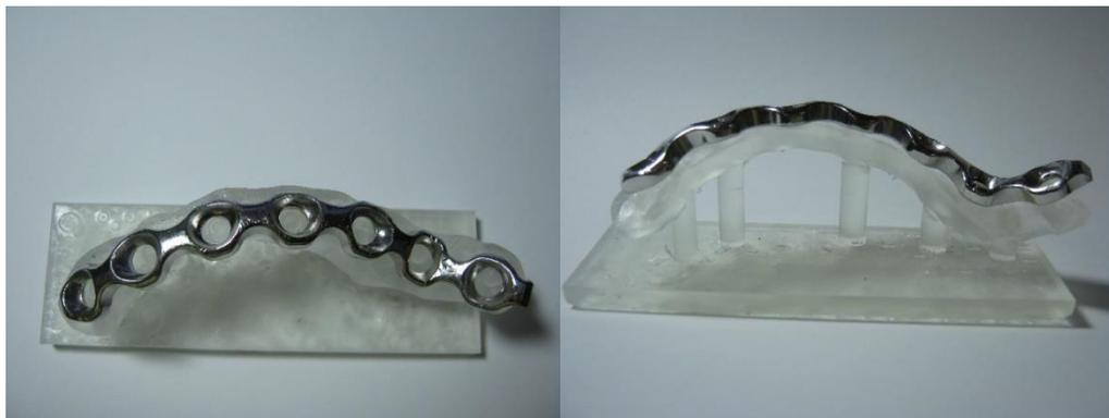
Figure 28 - Bending Template and Contoured Plate.
