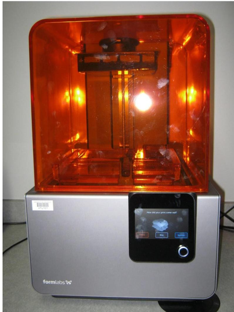
Figure 5 - Formlabs Form 2 Printer.
