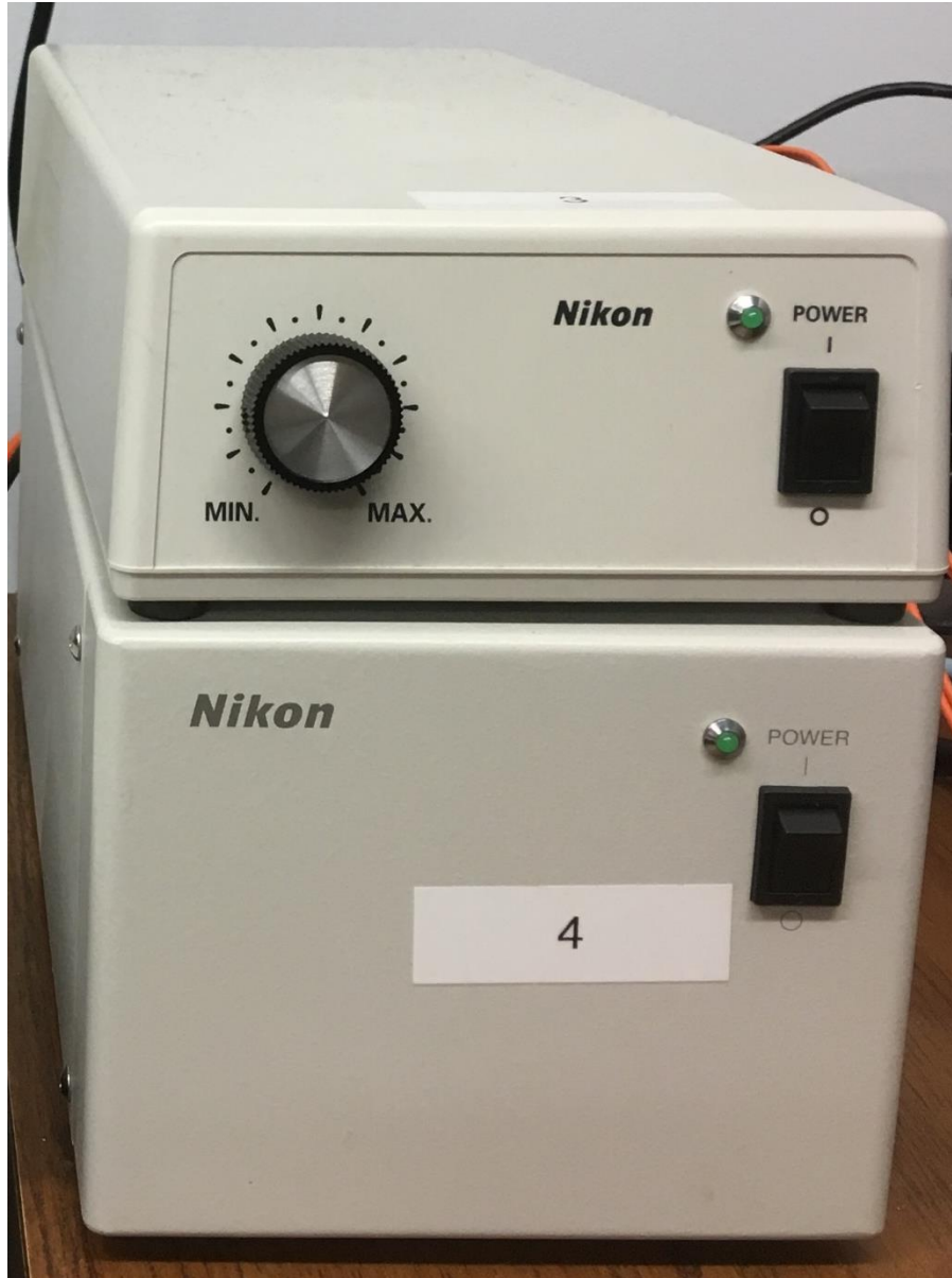
Figure 3. 29 Image of the LED light source for the confocal microscope (Nikon Eclipse Ti)
