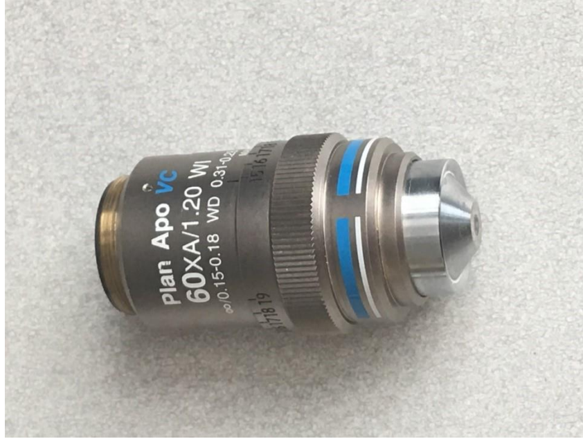
Figure 3. 21 Image of the Nikon 60× objective lens used in the laser trapping experiments
