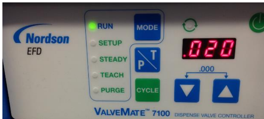
Figure 3. 5 Control panel display on the 3-axis robotic system with the dispense time for the valve controller displayed digitally in the upper right side of the image.
