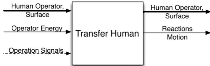
Figure 1. Black box model (Nagel, Bohm et al. 2015).
