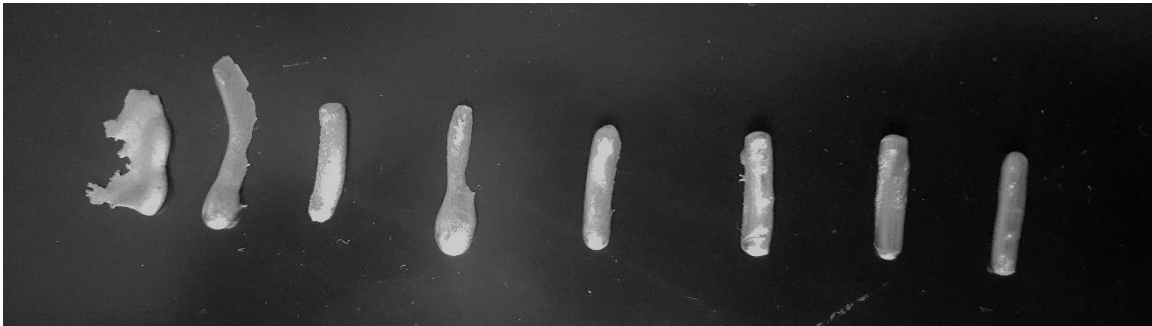
Figure A.4: Samples of the melted alloys over the temperature range of 135°C (left-most) to 170°C (right-most) at increments of 5°C.
