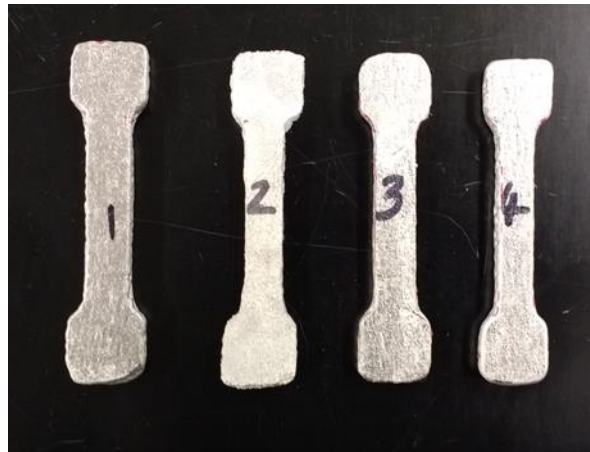
Figure A.15: Samples of Sn60Bi40_M2 as cast fabricated using the FFF casting methodology .
