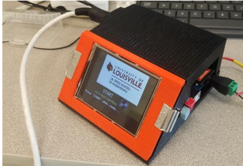
Figure 31 – Fully assembled device of printed parts enclosing device hardware
