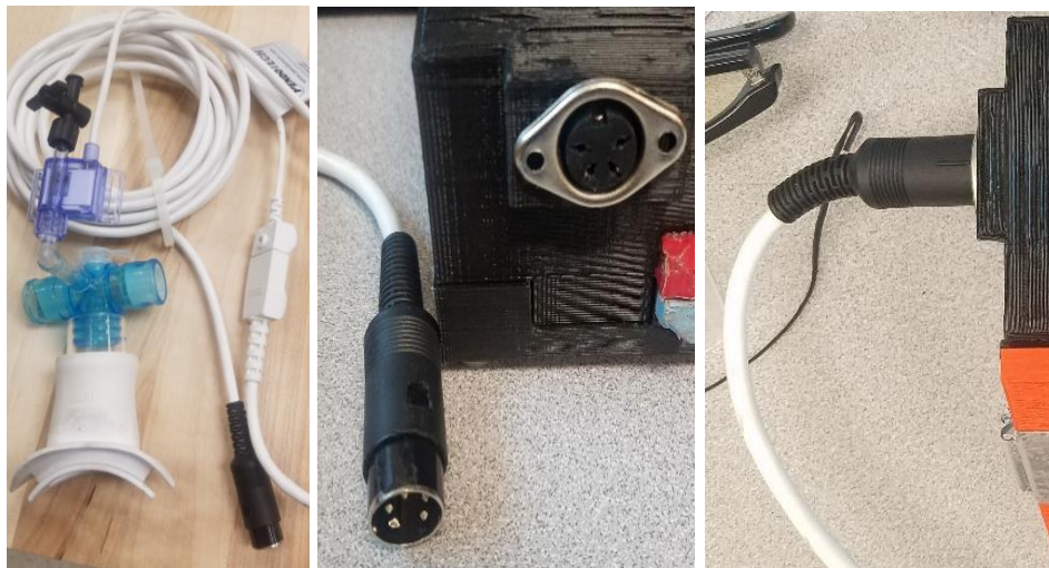
Figure 16 – (Left) Pressure sensor connected to male 4-pin connector. (Center) Male 4-pin connector and female 4-pin connector. (Right) Breathing apparatus (male) connected to BreathForce processing unit (female)
