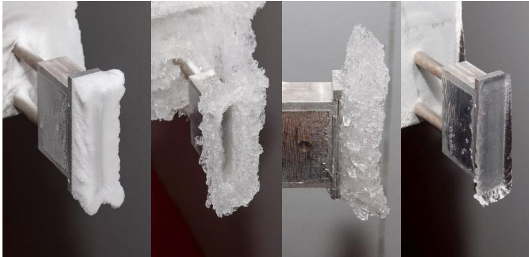
Figure 5. Types of aircraft ice. Left: rime ice (8/19/16 run 3), Middle: glaze ice (8/18/16 run 1), Right: Glaze (8/15/16 run 1). Photographs by Quentin Schwin.
