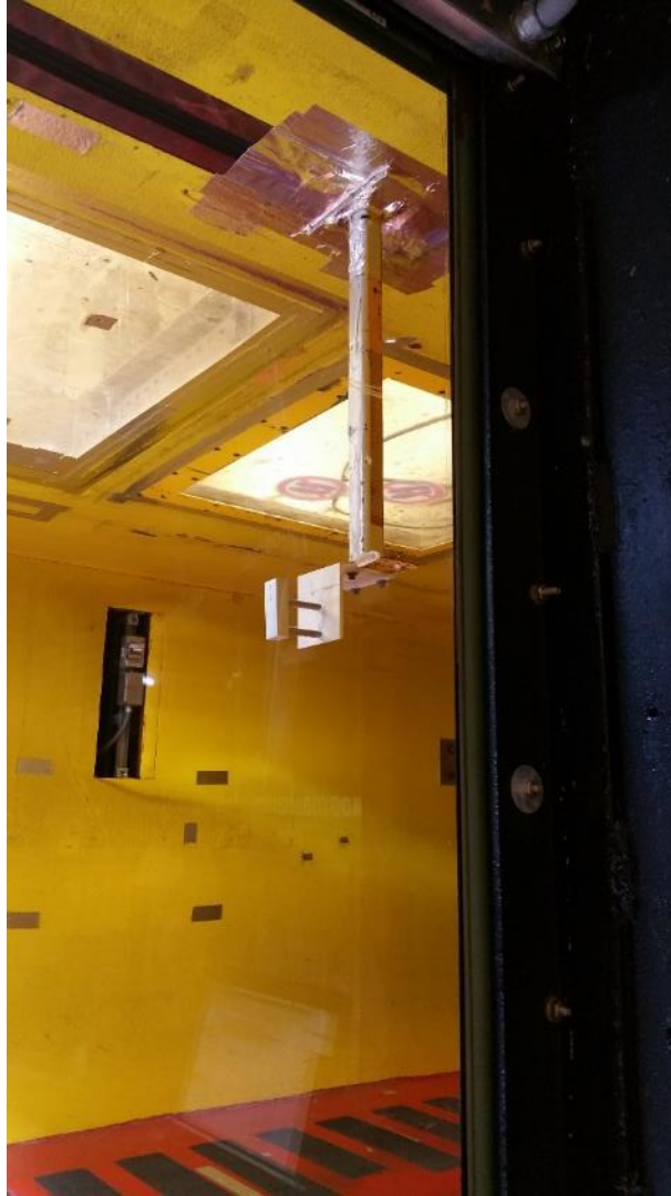
Figure 20. Test coupon mounted in the zipper slot of the IRT, aft of the primary test model.
