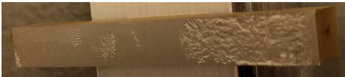
Figure 81. Surface cohesive break on sample AG15, post-test.
