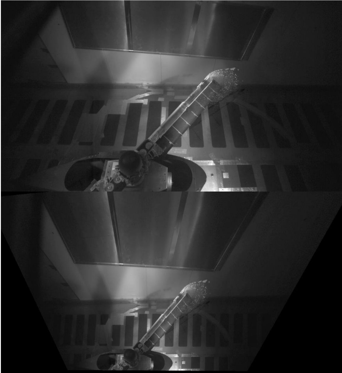
Figure 40. Top: Original image from Run 71. Bottom: Perspective corrected image.
