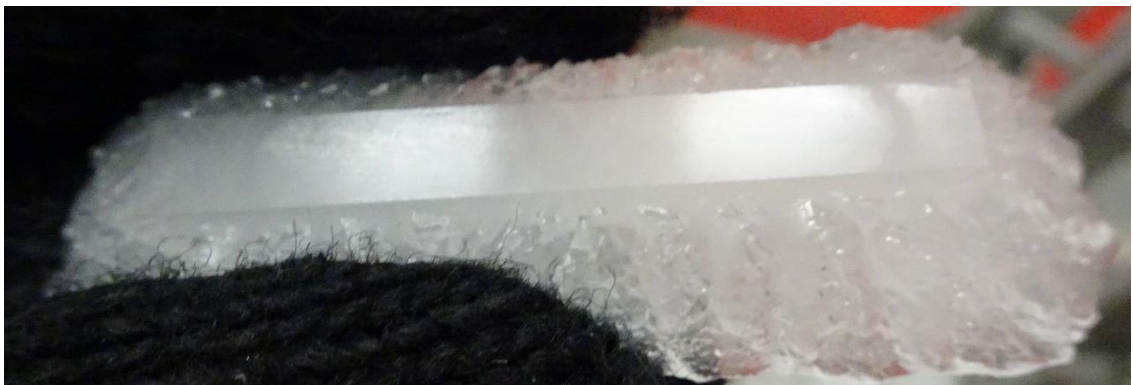
Figure 77. Sample delaminated during run AD showing marks near either end at ice-coupon interface.
