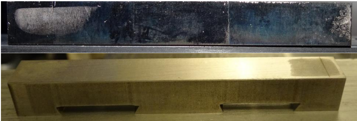
Figure 56. Frost on sample K11 (top) and W6 (bottom). Some frost sublimated before pictures could be taken.
