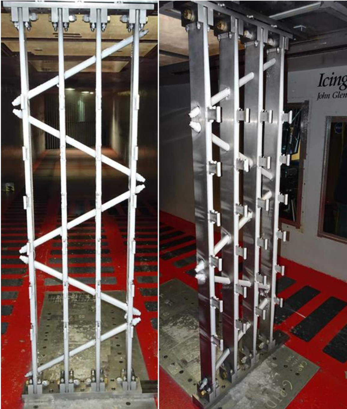
Figure 74. XT model in test section after run AJ, a rime condition.
