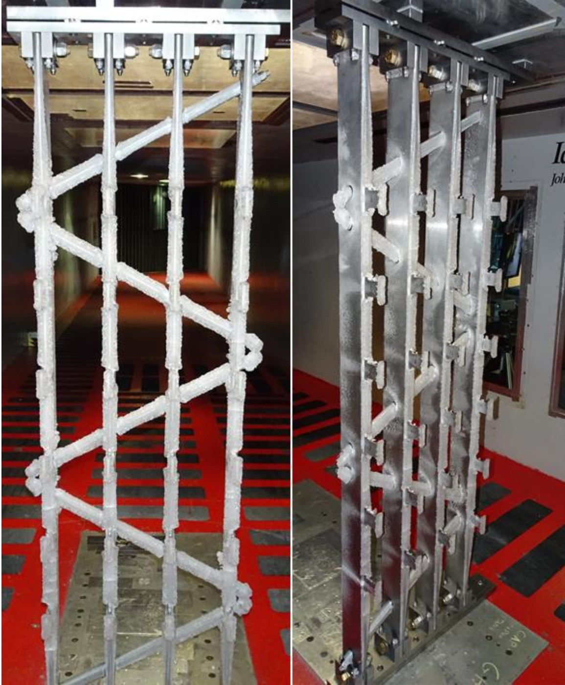
Figure 73. XT model in tunnel after run AB, a glaze condition.
