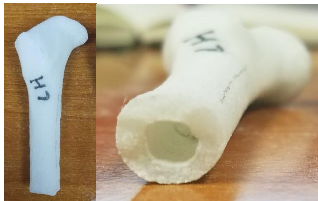
FIGURE 43. Sample fracture pattern of a hollow (labeled H7) as a result of three-point bending loads. Posterior view (left) and transverse plane view (right).
