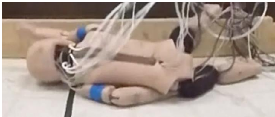
FIGURE 70. View of the initial impact of an ATD simulating a bed fall onto linoleum where the ATD had landed on its arm.
