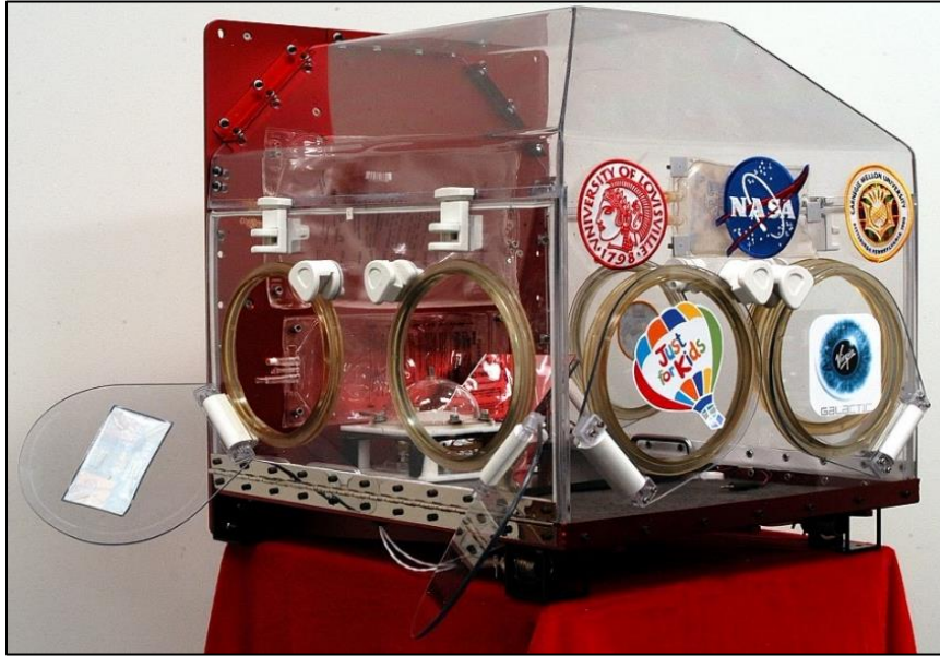
Figure 5 - Suborbital glovebox with polycarbonate canopy, incubator-style arm access ports, and absorbent liners situated underneath the two modular experiment boards
