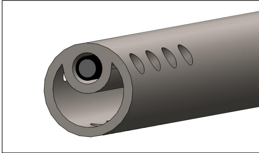
Figure 24 – Solid model of suction/irrigation wand distal tip showing dual-lumen design for fluid line and fiber optic cable (lumen outer diameter ~5 mm)
