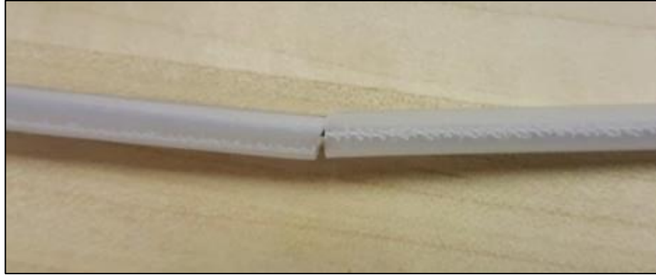
Figure 39 - Fracture in Accura 60 suction/irrigation wand
