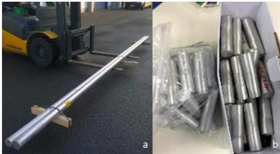
Figure 70 - Raw material (a – rod, b – reduced bolt)
