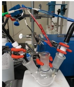
Figure 0.2. Electrochemical corrosion studies setup used in this study.
