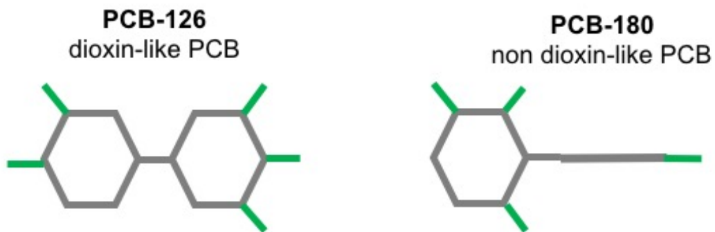
Figure 2. Chemical structure of PCB-126 (dioxin like PCB) and PCB-180 (non-dioxin like PCB): Figure 2 illustrates the chemical structure of PCB-126 (left) and PCB-180 (right). PCB-126 is co-planar and considered a dioxin-like PCB whereas PCB-180 is non-co-planar and considered a non-dioxin like PCB. Both PCBs have a carbon biphenyl ring structure (gray) with varying numbers of chlorine (green) and in various positions. The biphenyl rings for PCB-126 are in the same plane (coplanar) but PCB-153 have the biphenyl rings in different planes (non-coplanar) due to the positioning of the chlorine atoms.
