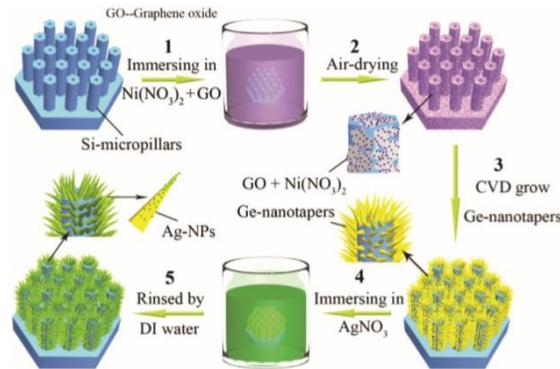
Figure 10- Schematic for the synthesis of Ag-NP@Ge-nanotapers/Si-micropillar hierarchical arrays. [Liu et al., 2015]
