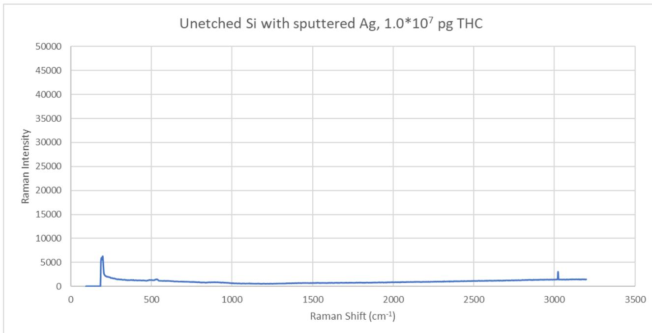
Figure 64: Bare Si chip, 10  $\mu\text{L}$  ( $1.0 \times 10^7$  pg) of THC on bare Si with Ag sputtered on
