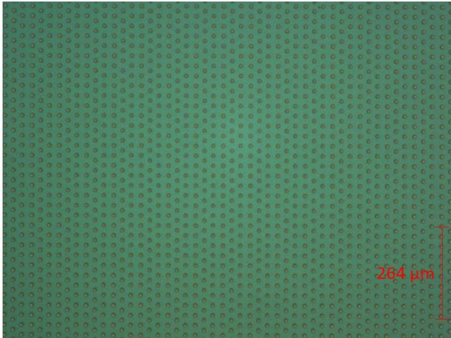
Figure 18: Photoresist pillars on Si, x5 magnification
