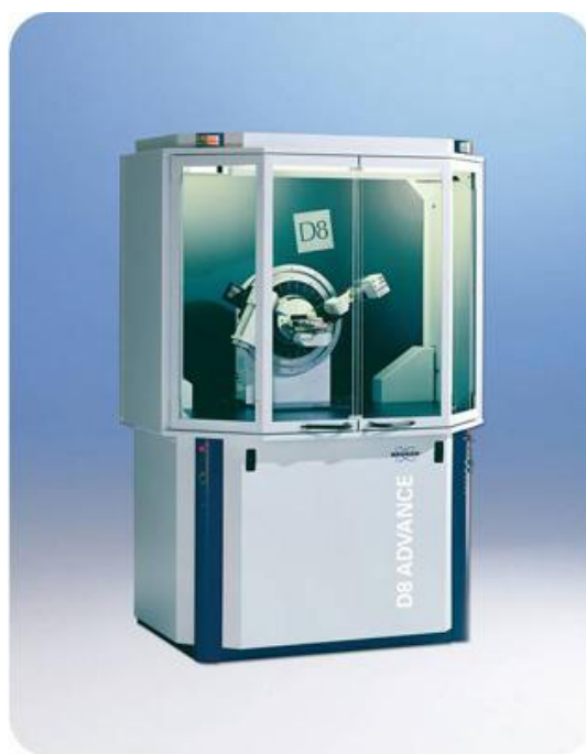
Figure 8. D8 Bruker Discover machine used for XRD characterization. For \text{Li}_6\text{PS}_5\text{Cl} , strong peaks are anticipated at 2\theta=25.3 , 29.9 , and 31.3^\circ .
