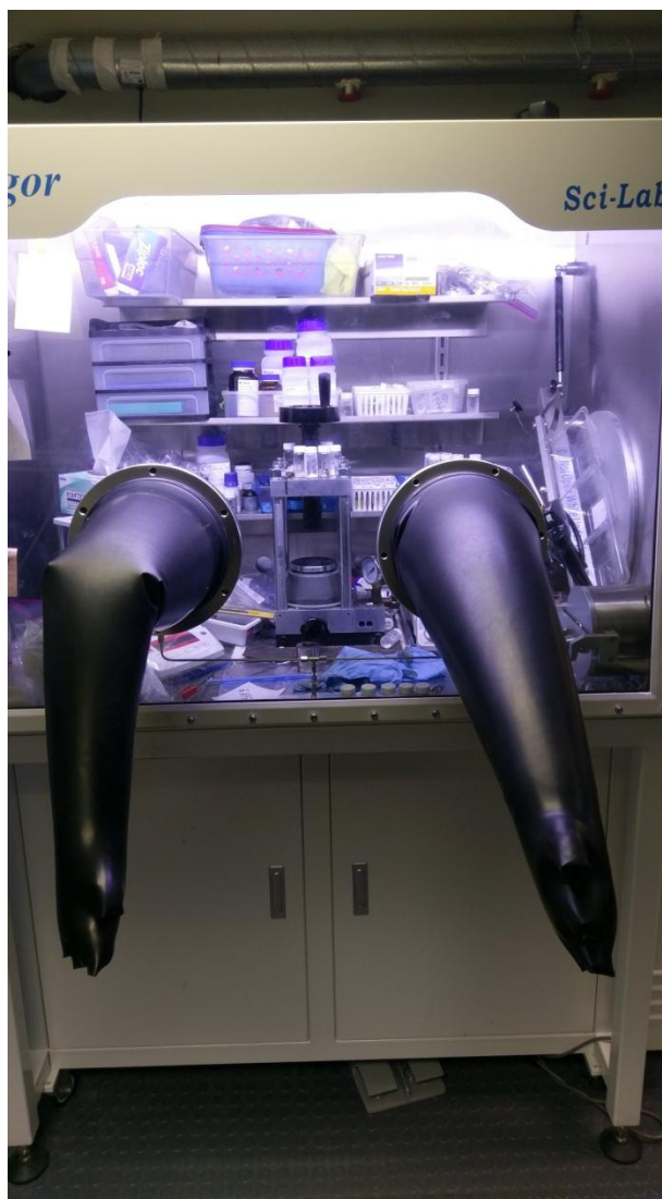
Figure 6. The primary glovebox used for materials preparation. It is filled with inert argon gas, and controls oxygen and water levels to under 1 ppm. The hydraulic press inside was used to densify solid electrolyte powder into thin pellets.
