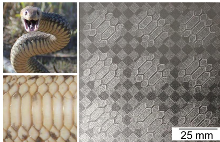
Figure 6.8 Snake skin-inspired patterns in 420 stainless steel fabricated by L-PBF for potential use in wear resistant moving parts.
