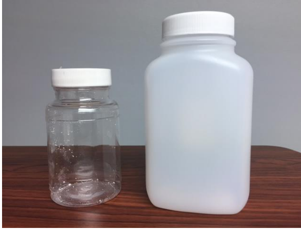
Figure 24. (left) E. coli bottle (120 ml) with chlorine-neutralizing agent, (right) TSS bottle (250 ml).
