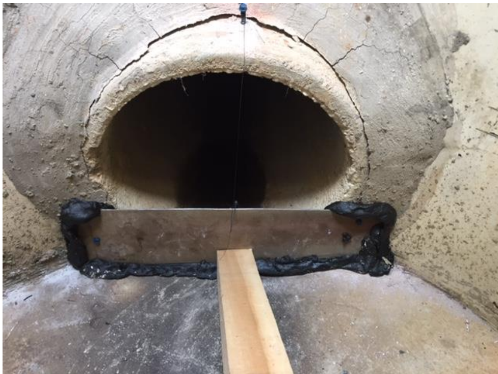
Figure 20. The weir installed in front of the headwall in UGF-1.
