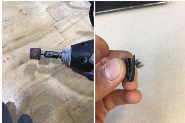
Figure 37: Image of the Dremel tool (left) used to taper the arms of the device (right).
