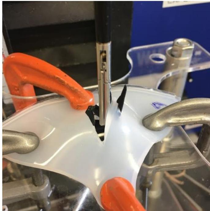
Figure 87: Broken Acetone treated device during delivery into dragon skin silicone.
