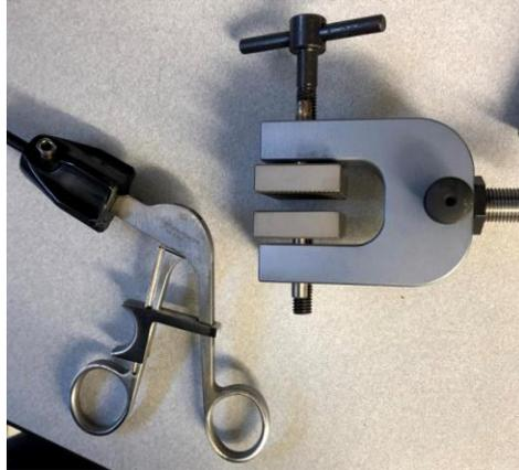
Figure 62: Clamp placed onto Snowden-Pence Lap Tool.
