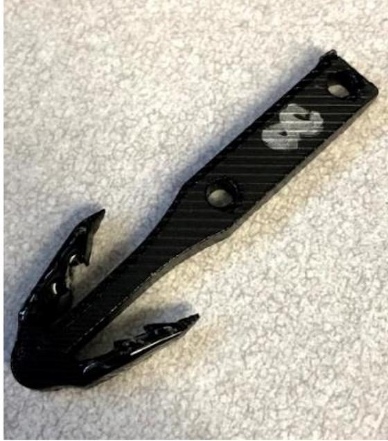
Figure 47: Drops of acetone on arms of the device to soften the PLA material.
