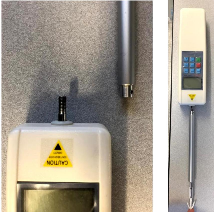
Figure 60: The attachment of the applicator to the hand-held force gauge.
