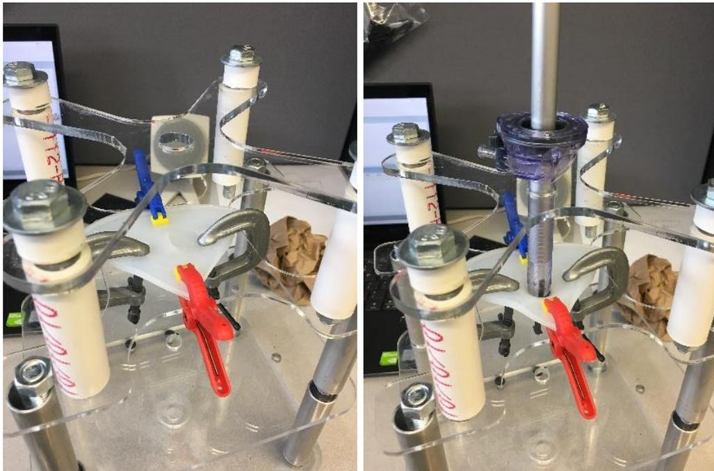
Figure 51: Visual of test set-up before (top) and after (bottom) of trocar in and out of test fixture.
