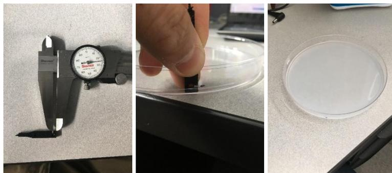
Figure 55: Measurement of petri dishes and pouring silicone into petri dishes.
