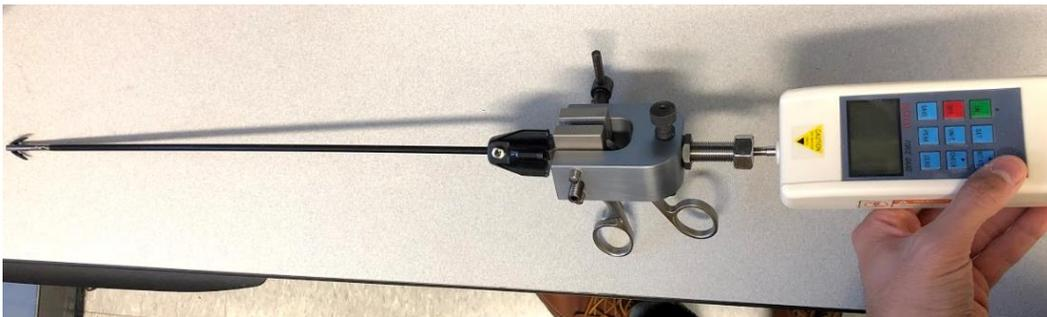
Figure 63: Attachment of clamp to hand-held force gauge depicting entire set-up for cadaver testing.
