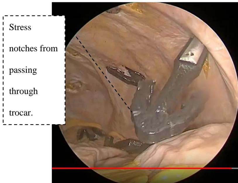
Figure 90: Picture of the "Previous" Device in cadaver abdominal cavity before delivery.
