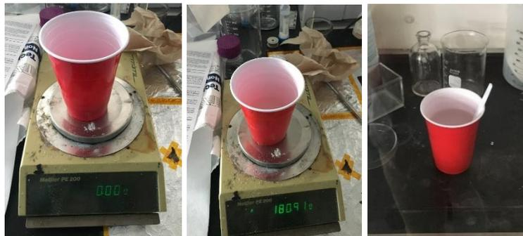
Figure 54: Weighing of mixture components (left and middle) and mixing of components in fume hood (right).
