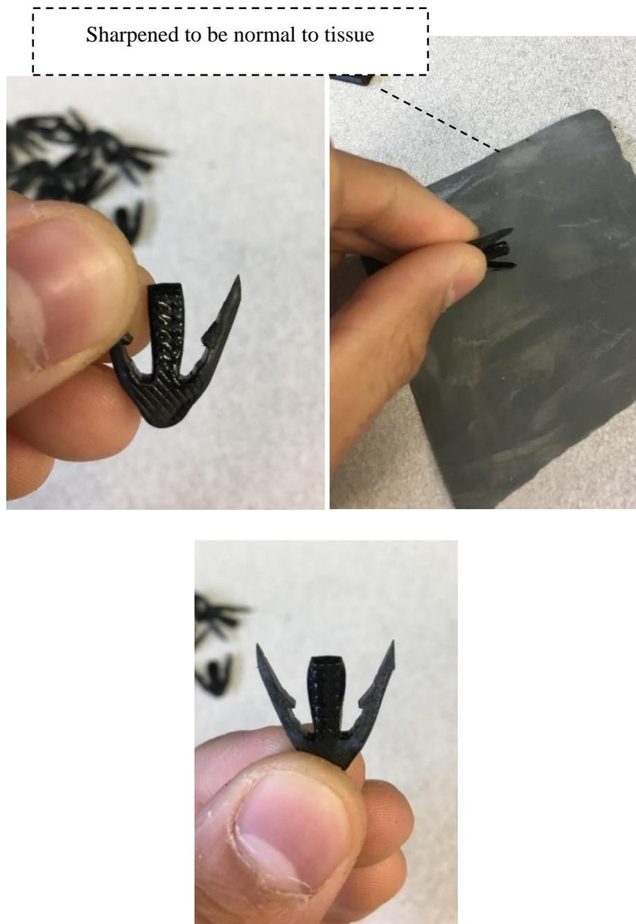
Figure 40: Final sharpening with grade P1600 sand paper of device arms: Top left: before sanding; Top right: sanding process; and, Bottom: finished device.
