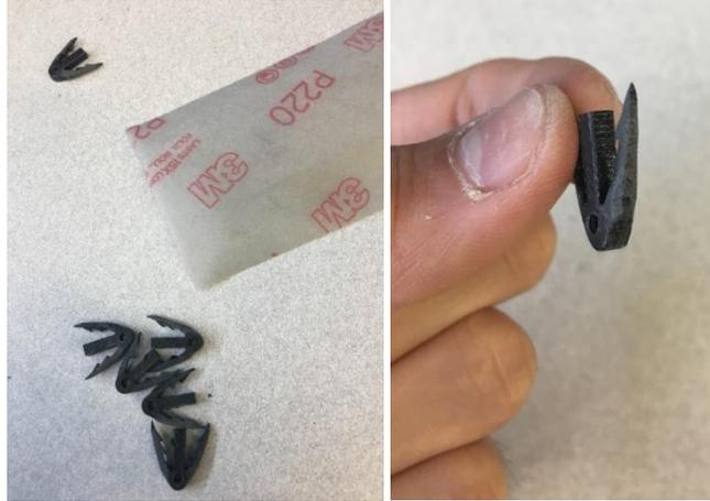
Figure 38: Image of device arms sanded with P220 grade sand paper for smooth finishing.
