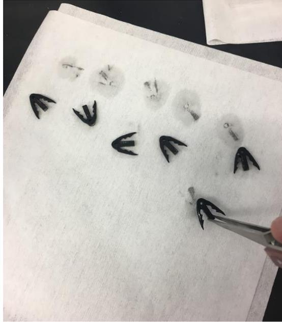
Figure 57: Acetone treated devices drying.
