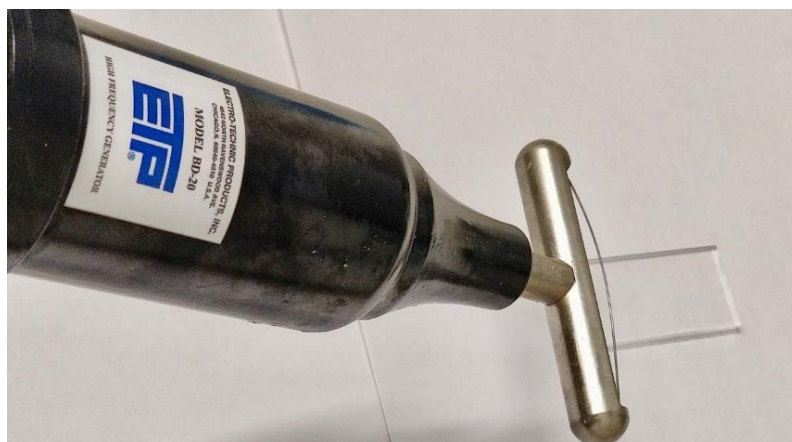
Fig. 3. 8 Corona treatment on the PMMA samples just before adding the solvent to the samples
