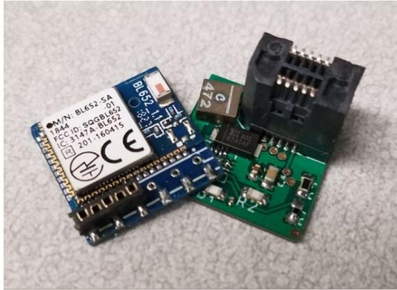
Figure 15. Shows the final electronic backpack assembled. The board on the left houses the microcontroller and necessary UART connections. The board on the right is the bottom board which contains power components including the voltage booster.
