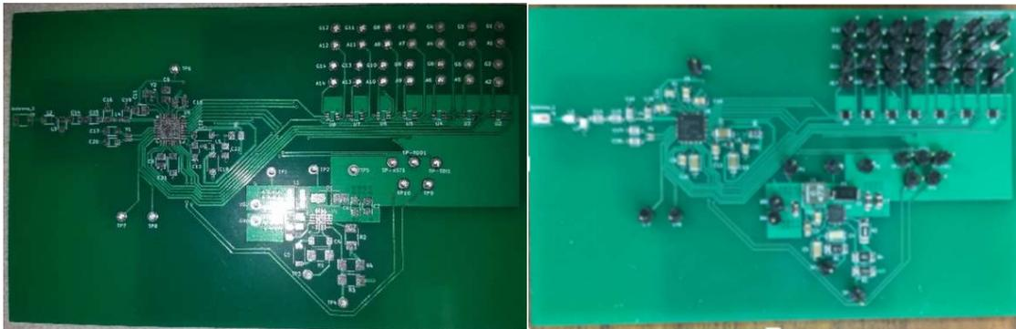
Figure 2. Shows ARRIPede V2. Left) Pads only. Right) Fully Assembled [39].
