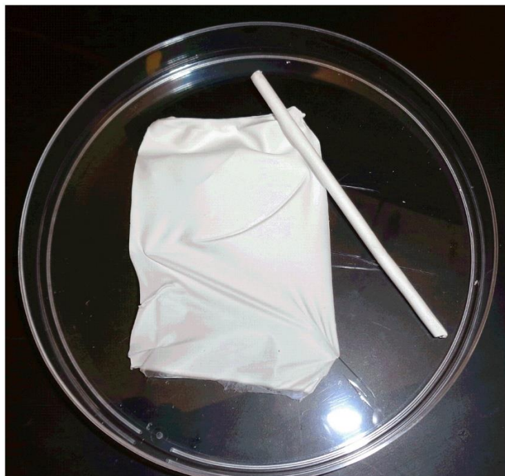
Figure A.1 The macroscale morphology of electrospun fibers. The electrospun fibers shown were fabricated using a 4 mm (cylinder) and 25 mm (sheet) diameter mandrel, respectively.
