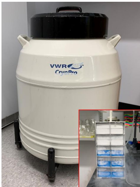
Figure 3. 18 Image of VWR CryoPro liquid nitrogen tank and the insert image shows the drawers in a rack system inside of the tank
