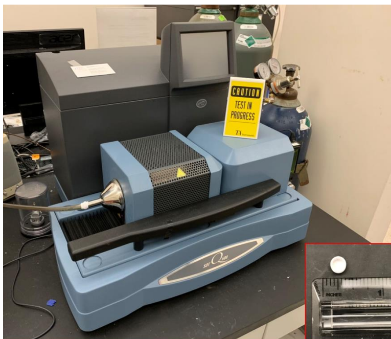
Figure 3. 9 Image of TA SDT Q600 Simultaneous TGA/DSC. Inserted image shows the ceramic cup that holds the sample
