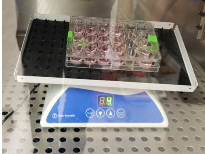
Figure 3. 31 Cells seeded on the scaffold with slow rocking on a rotating mixer in the incubator
