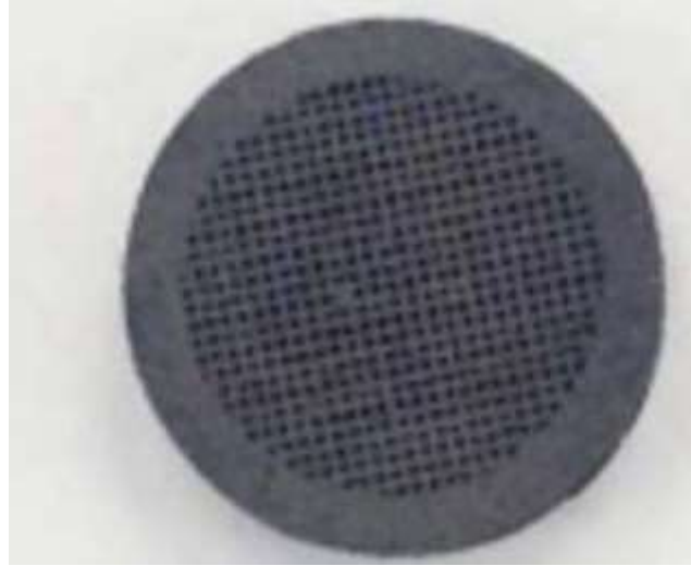
Figure 7: Microchannel regenerator example from Oak Ridge National Labs (Momen, 2017).
