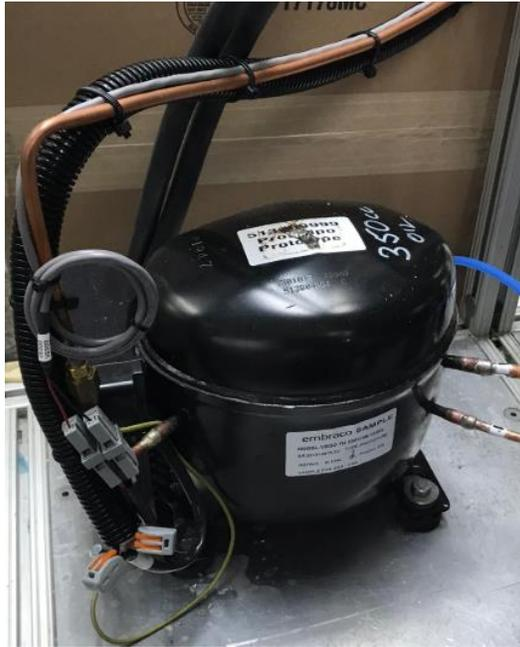
Figure A3 Embraco VEGD 7H mounted to forward heat leak calorimeter fixture
