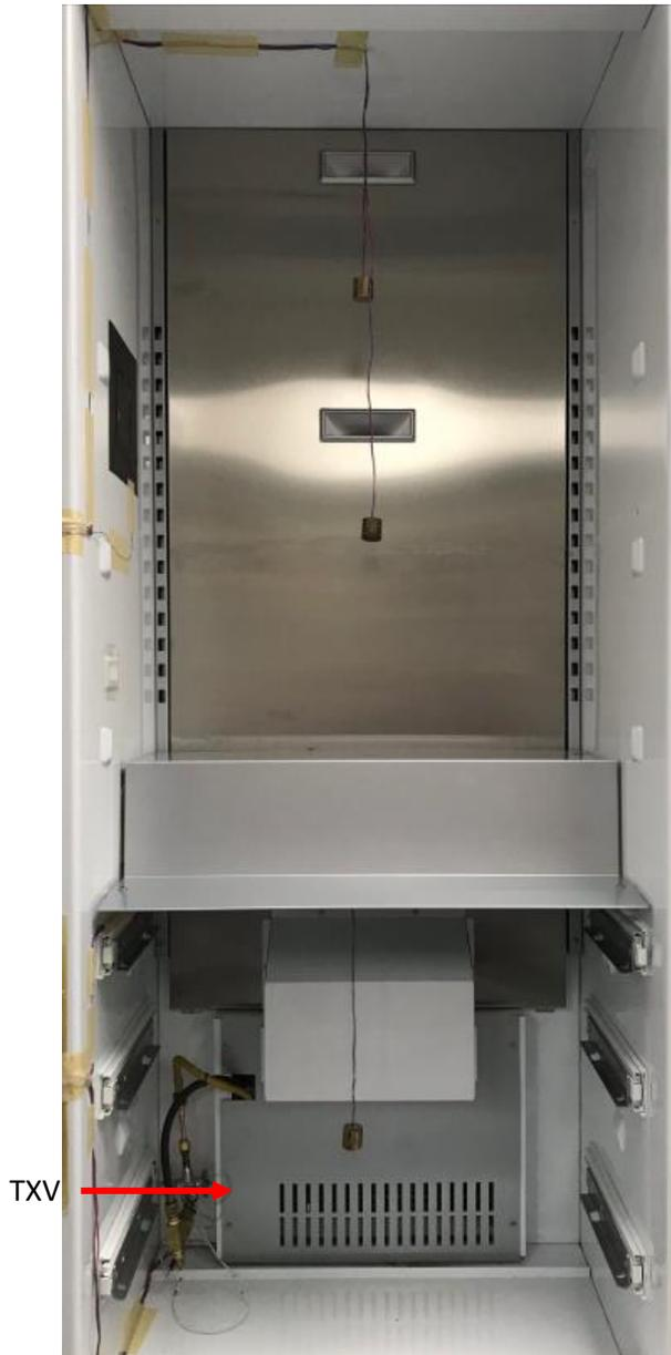
Figure A8 Front view of unit with TXV and evaporator cover installed
