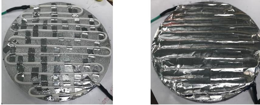
Figure 2-5 Aluminum plate with coil heater adhered to its bottom surface
