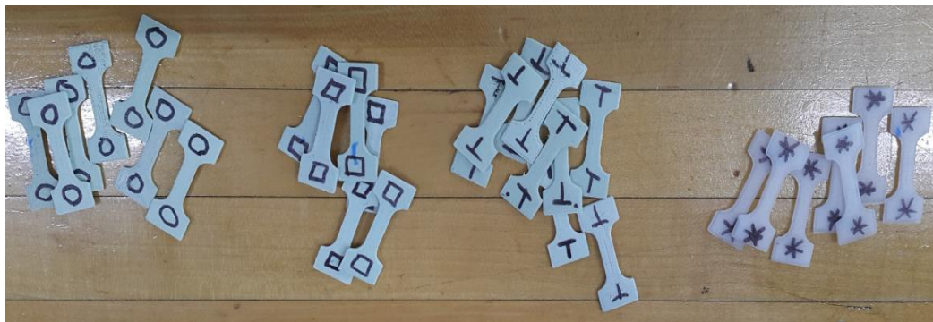
Figure 46. Fabricated samples via MEAM process, from left to right composite 10% fill (○), composite 2.5% fill (□), composite 1% fill (△), and homopolymer PVDF (*).
