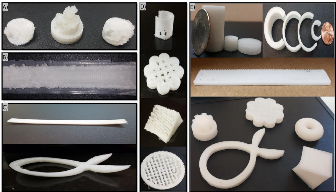
Figure 6. Printed PVDF parts experiencing poor dimensional accuracy(A), poor surface finish on perimeters(B), deposition bed delamination(C), and poor inter-layers bonding quality(D), contrasted with similar parts fabricated under viable printing parameters(E)
