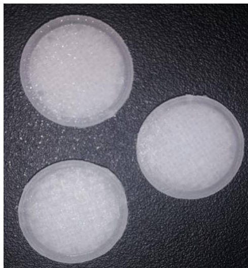
Figure 9. PVDF samples for electro-mechanical test
