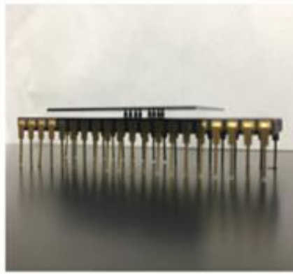
Figure 5-12 Assembled and packaged SolarPede die carrying a payload.
