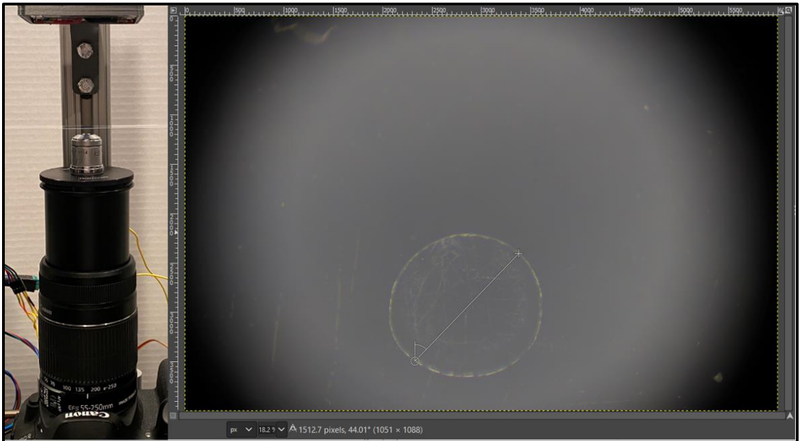
Figure 25. Uncropped image of droplet using 4x objective lens mounted to a telescopic lens to account for mechanical tube length of objective.
