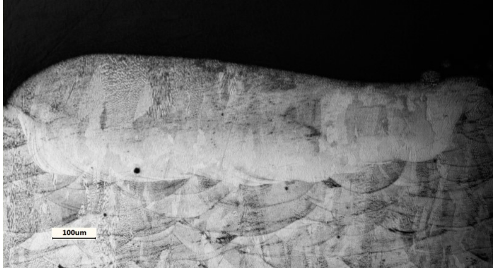
Figure 9.12 Longitudinal melt profile obtained with 195 W and 400 mm/s.
