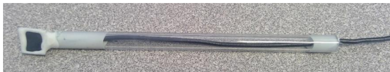
Figure 6. Example of an epoxied electrode. The active surface area on the left side is defined by the applied epoxy.
