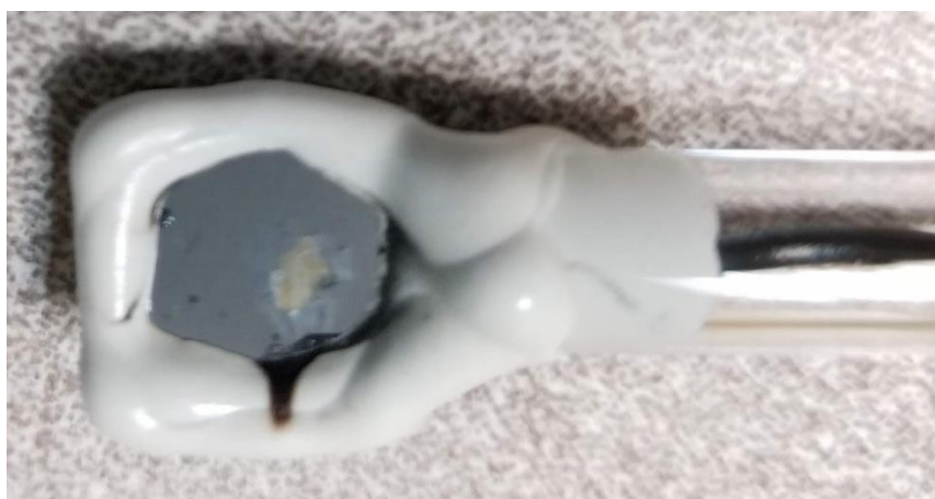
Figure A7. Delamination of BDD film on a tungsten substrate after extended use.
