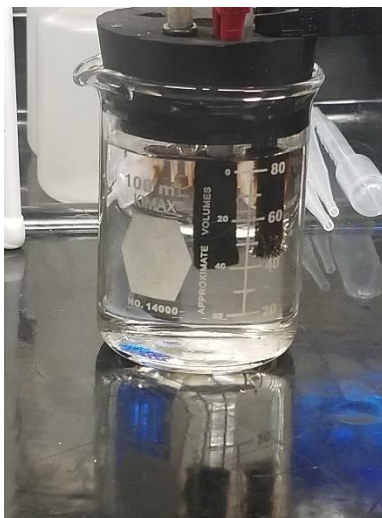
Figure A4. Three-electrode setup using a beaker, rubber stopper, graphite felt working and counter electrode, and Ag/AgCl reference electrode.
