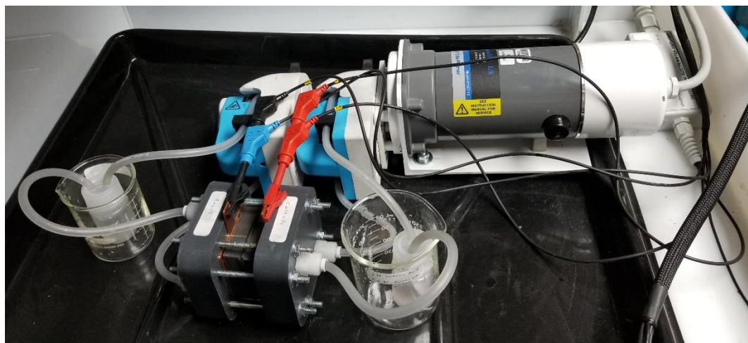
Figure 9. Full RFB testing setup complete with two storage reservoirs and a peristaltic pump.
