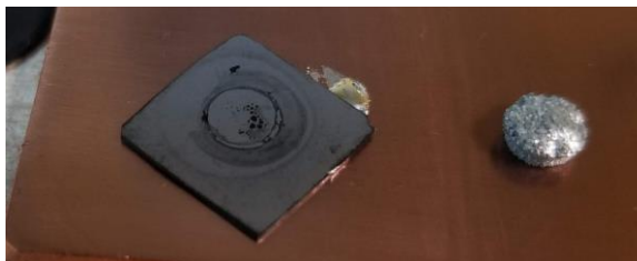
Figure A12. A zinc pellet formed as a result of electrodeposition on a BDD electrode.
