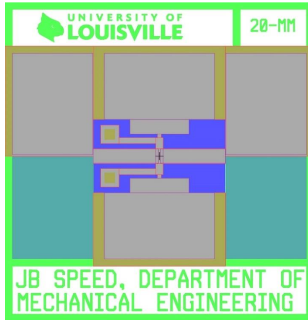
Figure 51. All five photomask layouts superimposed on the top of another.
