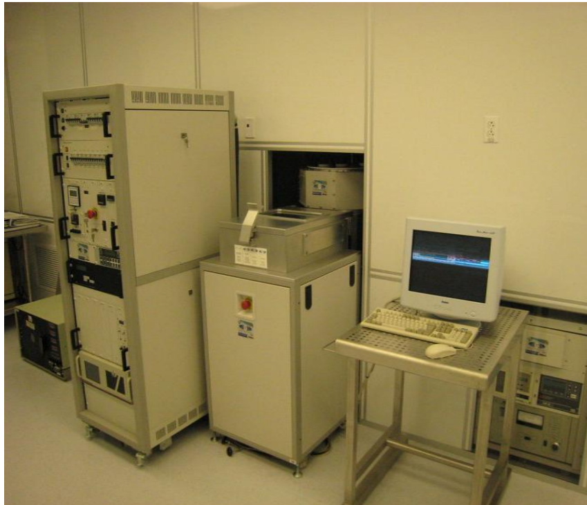
Figure 61. Deep reactive ion etching (DRIE) machine located in the etching bay at the UofL Micro/Nano Technology Center.
