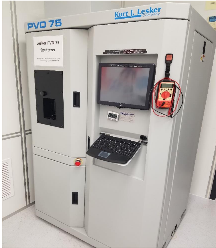
Figure 58. Kurt J. Lesker PVD 75 Sputtering machine located in the deposition bay at the UofL Micro/Nano Technology Center.
