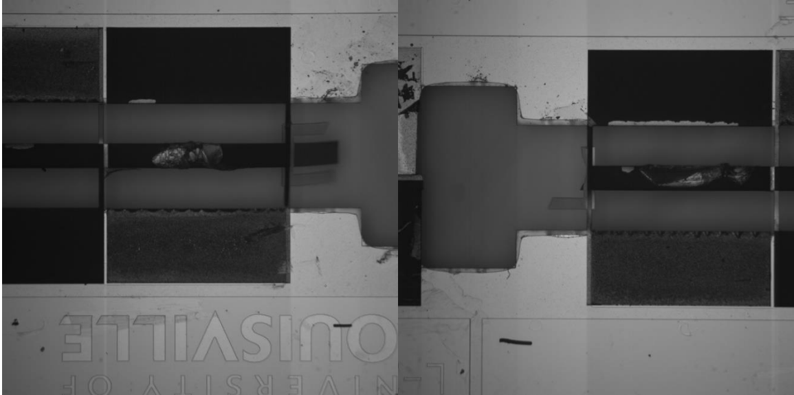
Figure 67. Microscopic pictures of the designed extended version of the bistable energy harvester after the final release.
