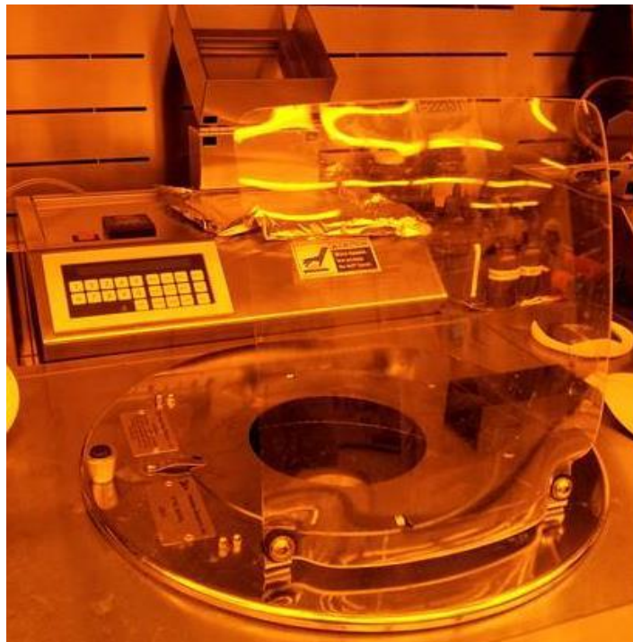
Figure 52. The Headway Spinner and the hotplate located in the photolithography bay at the UofL Micro/Nano Technology Center.
