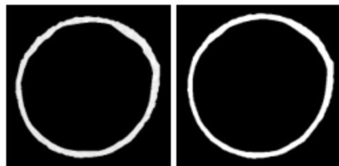
Figure 31: The original gray image of cortical bone on the left converted to binary image on the right in ImageJ
