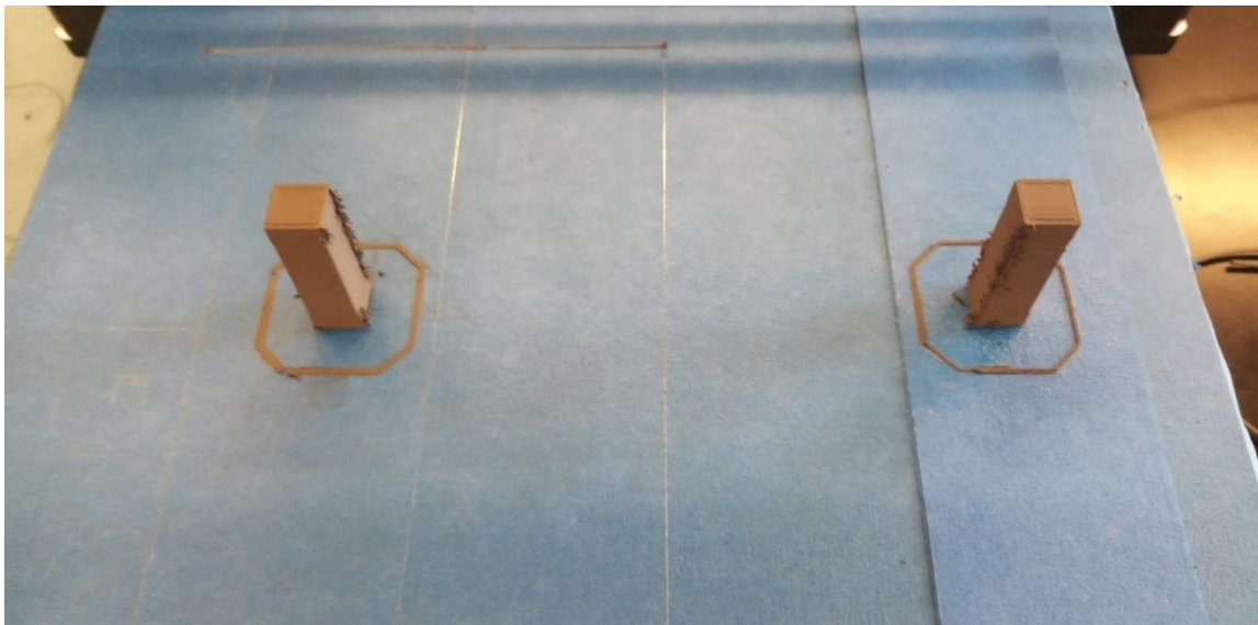
Figure C-II.4. Two square bars placed at a distance were chosen as test specimen to allow sufficient time for clear reading of the latest layer temperature and evaluate temperature drop between two layers
