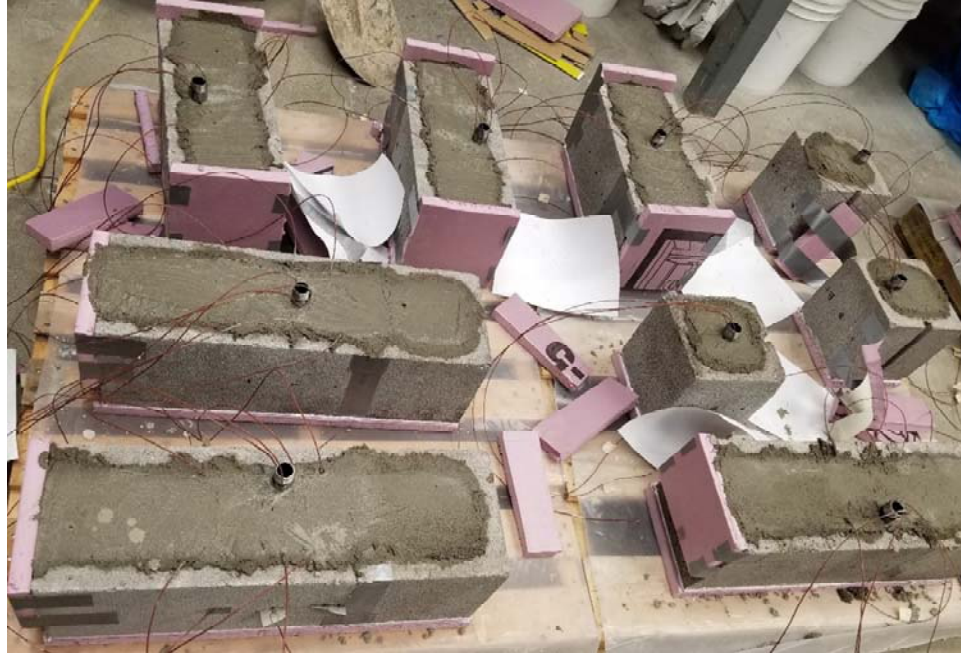
Figure 4-5 Specimen Casting (Active Thermal Insulation Wall Specimen)
