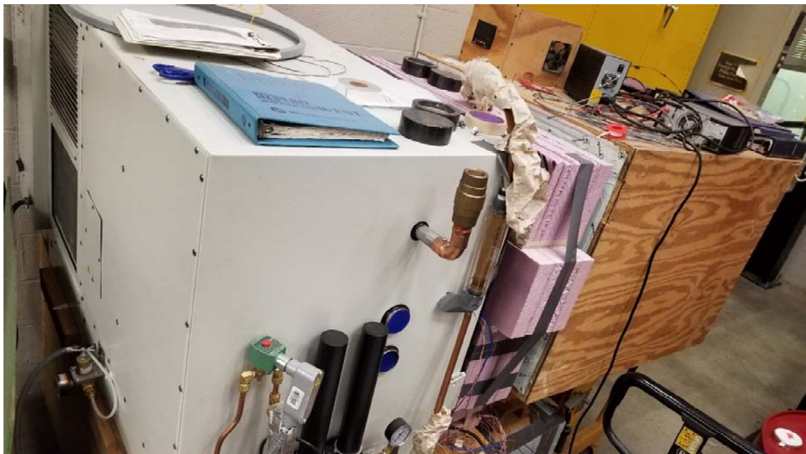
Figure 4-10 Hot Box Test Apparatus Demonstration
