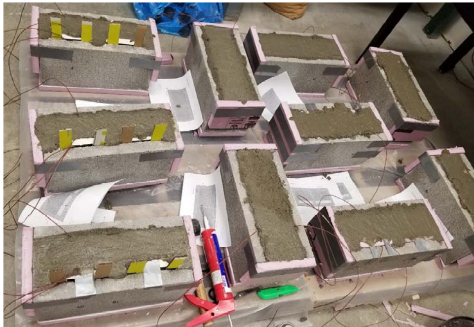
Figure 4-4 Specimen Casting (Conventional Wall Specimen)
