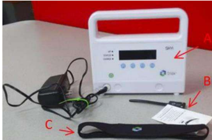
FIGURE 18 – (A) SKYi aggregator receiver with power cord; (B) SIM G; (C) Headband
