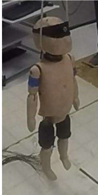
FIGURE 21 –SIM G placement on 12-month-old CRABI ATD
