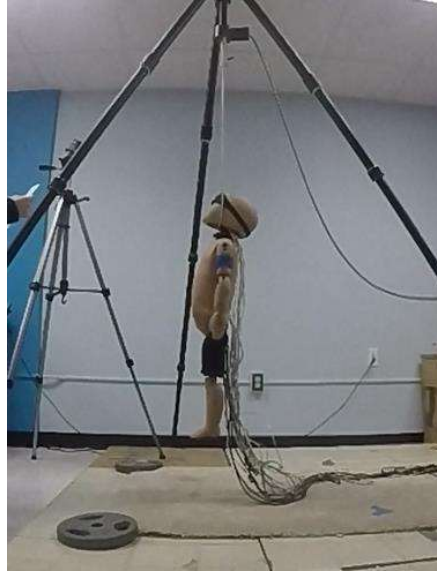
FIGURE 20 – Experimental test set-up for 0.69 m fall to verify SIM G
