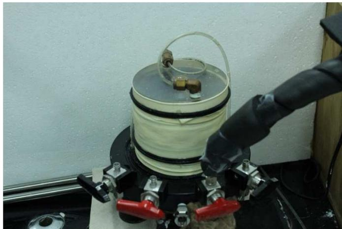
*Figure 0-1 Kalin sample placed on the base plate and covered by a latex membrane*
