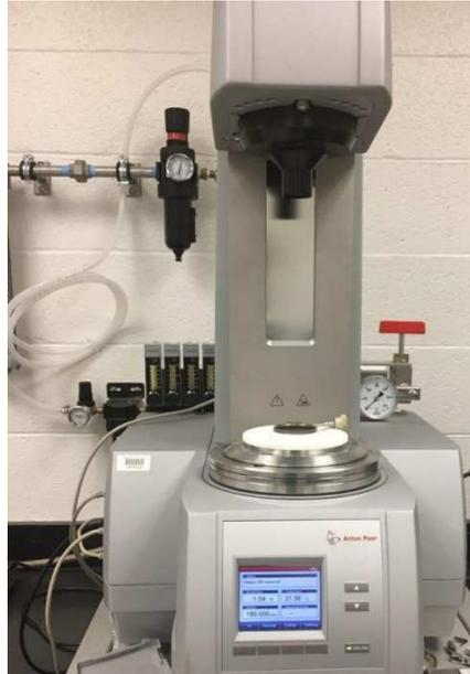
*Figure 3-6 Rheometer used to measure the dynamic viscosity of water at different temperatures*
