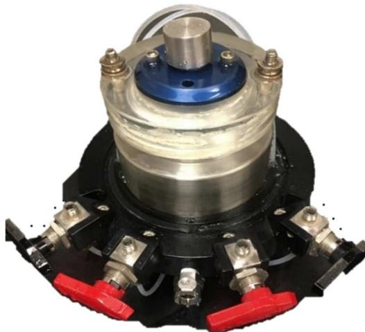
Figure 4-3 Consolidometer and the sample inside it on the base plate
