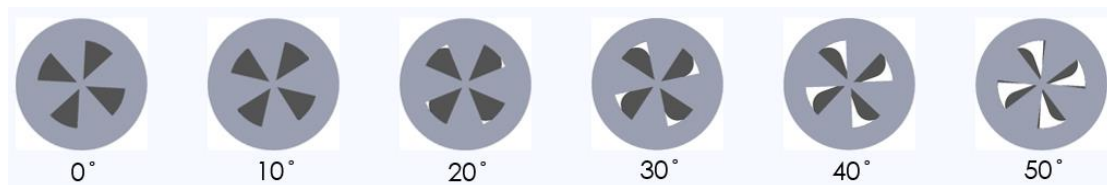
Figure 3.7 – A proportional valve design in SOLIDWORKS is moved from completely closed to completely open using an angle mate.
