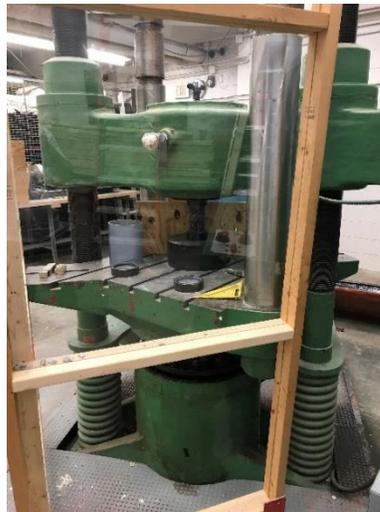
**Fig. 2.13.** Universal compression testing machine with the load range to 400 kips
