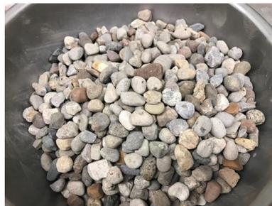
**Fig. 2.2.** 0.9525 ~ 1.27 cm (3/8 ~ 1/2 in.) rounded aggregates
