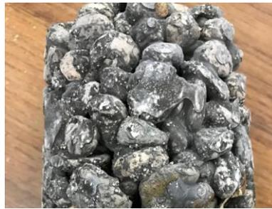
**Fig. 3.13.** MGPC sample with PM-199 replacement of cement
