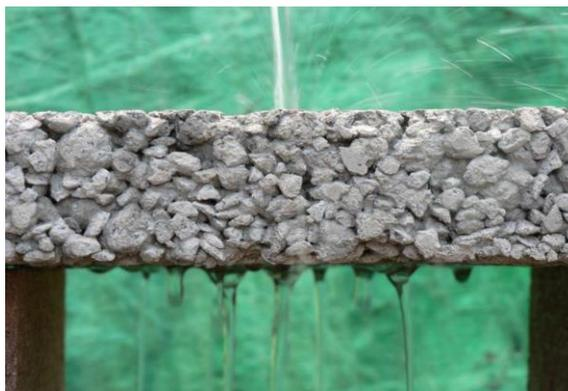
**Fig. 1.3.** Conventional pervious concrete (Ready Mixed Concrete Association)
