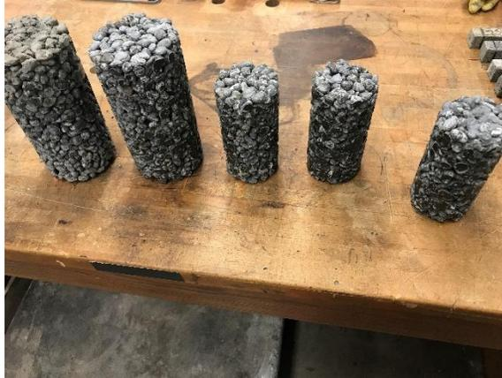
**Fig. 2.12.** Sample preparations of pervious concrete with different sizes
