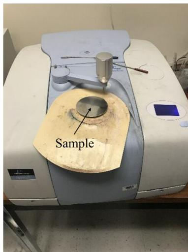
**Fig. 4.2.** PerkinElmer Spectrum 100 and FT-IR Spectrometer
