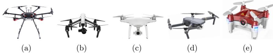
Figure 13: UAVs from (a) DJI Matrice 600 Pro, (b) DJI Inspire 1 Pro, (c) DJI Phantom 4 Pro, (d) DJI Mavic Pro 1, (e) Beebeerun. The UAVs considered include medium, small and mini size.
