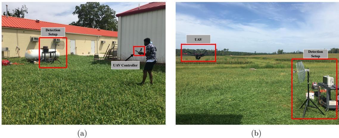
Figure 18: The RFSSCS setup for visual line of sight capturing of signals from : (a) a UAV controller, (b) a UAV (DJI Matrice 600).
