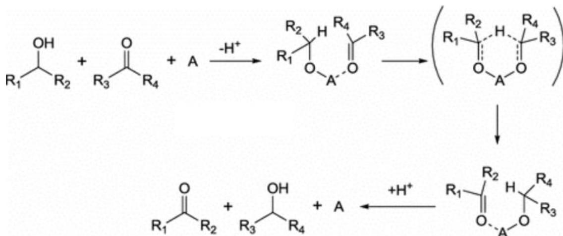
FIGURE 1 – MPV Reduction Mechanism. From Nakagawa, Y., et al. (2018). "Perspective on catalyst development for glycerol reduction to C3 chemicals with molecular hydrogen." *Research on Chemical Intermediates* 44: 1-25.
