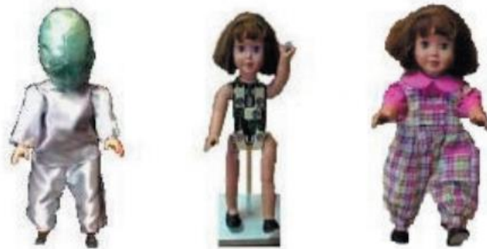
Figure 2. Robota robot, left is the obscured robot, middle shows the robotic parts, and right is the dressed robot [1]
