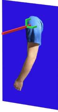
Figure 46. Normal to the plane formed by V_{se} \times V_{eh}
