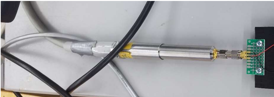
Figure 2. Image of the 42941A Impedance Probe attached to the fabricated chip holder
