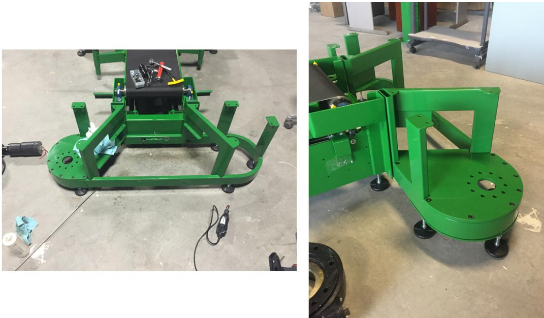
Figure 4.31: Modular Back Deck Install (Left) and Back Deck Leveling Feet with Crane Plate (Right)
