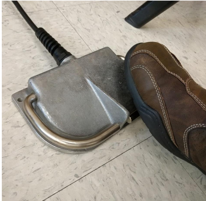
Figure 3.67: Slew Ring Control Switch
