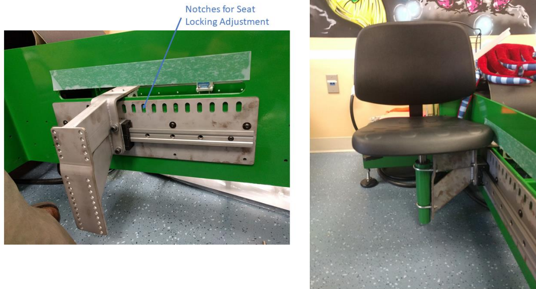
Figure 4.28: Rev. 3 Cantilever Side Seating Arm (Left) and Installed Rev. 3 Side Seating (Right)
