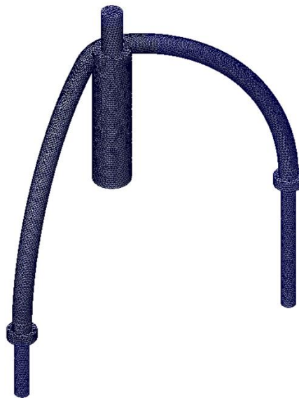
Figure 3.37: Mesh Density of Trunk Trainer Seat FEA
