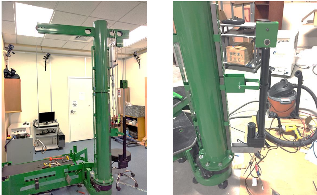
Figure 4.35: Fully Assembled Crane (Left) and BWS Support Brackets and Pulley Brackets (Right)
