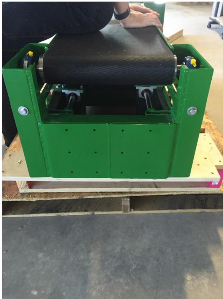
Figure 4.16: Rear View of Treadmill Showing Open Back End and Roller Tensioning Bolts
