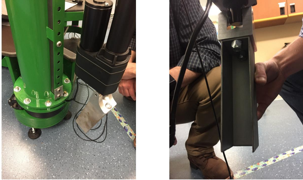
Figure 4.45: Rev. 1 Cylinder Support Box Bracket Failure
