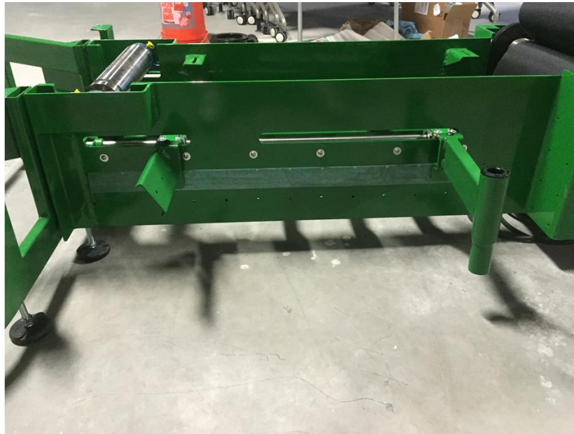
Figure 4.17: Installed Rev. 1 Footrest Arm and Rev. 1 Side Seating Arms
