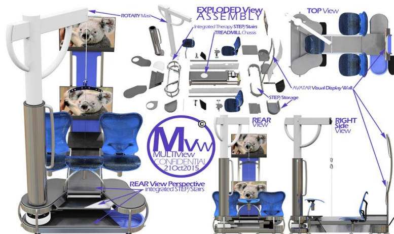
Figure 3.3: Concept Rendering of Beta Prototype Showing Modularity and Symmetry
