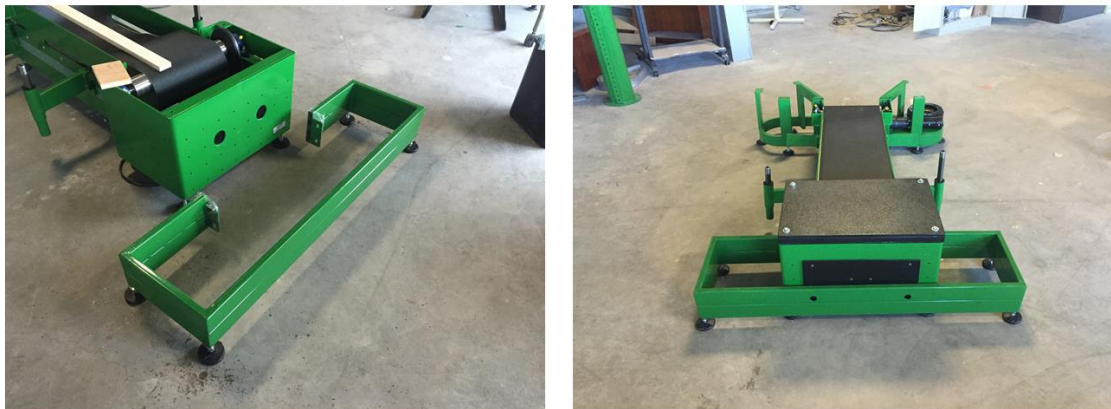
Figure 4.30: Modular Front Deck Install (Left) and Installed Front Deck (Right)
