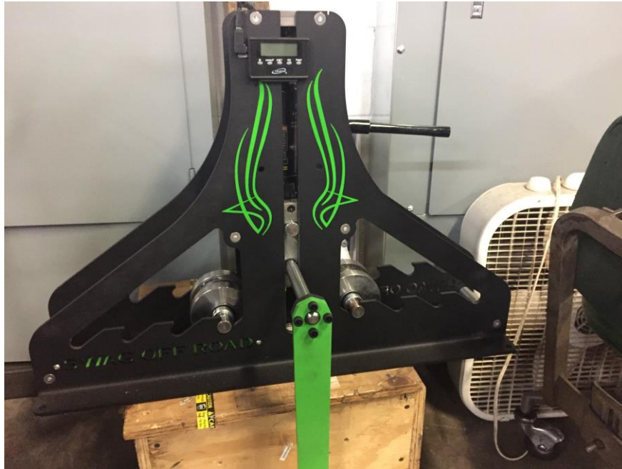
Figure 3.49: Tube Bender for Support Struts on Rear Deck
