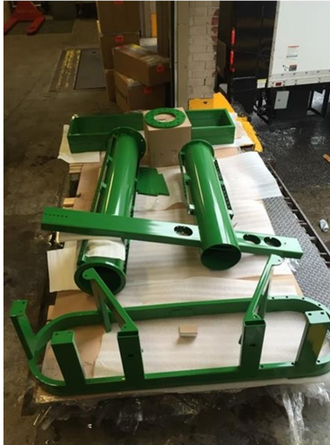
Figure 4.8: Shipping Pallet Containing Top/bottom Crane Mast, Back Deck, Front Deck and Crane Plate
