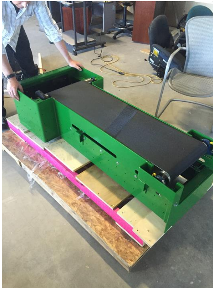
Figure 4.9: Assembled Central Treadmill
