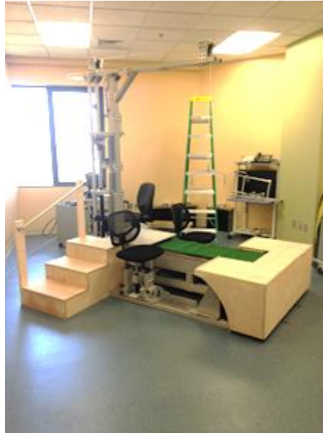
Figure 2.9: Fully Functional Prototype of Alpha Unit Pediatric BWST
