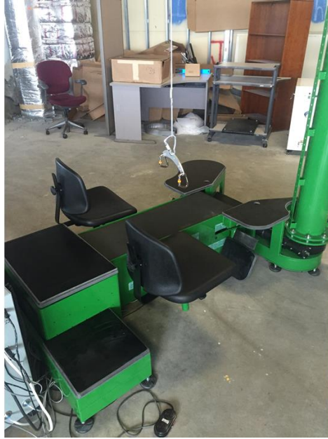
Figure 4.18: Assembled Rev. 1 Right and Left Side Seats and Rev. 1 Footrests
