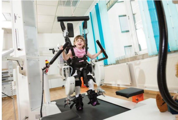
Figure 2.5: Lokomat with pediatric add-on module
