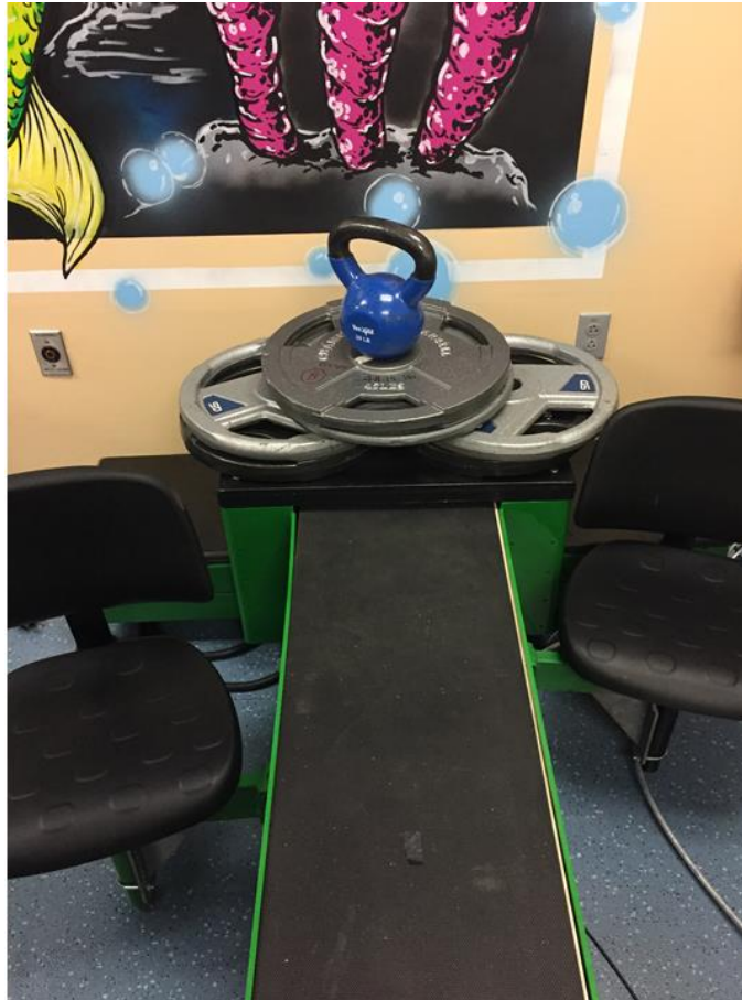
Figure 4.15: Weight Testing of Motor Housing - 309.96 lbs. (E, F, G, H, I, J, K) for 10 mins.
