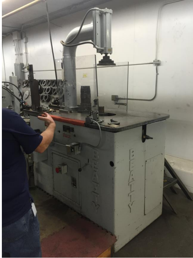
Figure 3.47: Beatty Tube Bending Machine at Winston Industries
