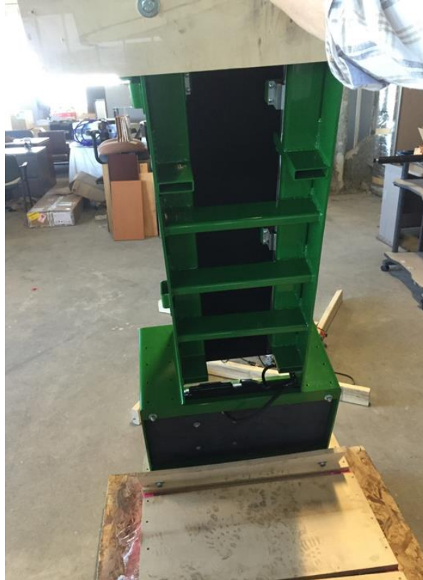
Figure 3.21: Treadmill bottom view – note internal crossbeam supports
