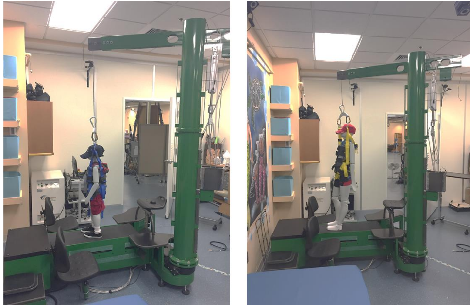
Figure 4.4: Complete BWST System with 3' 3" Child Manikin (Left) and 4' 9" Child Manikin (Right)
