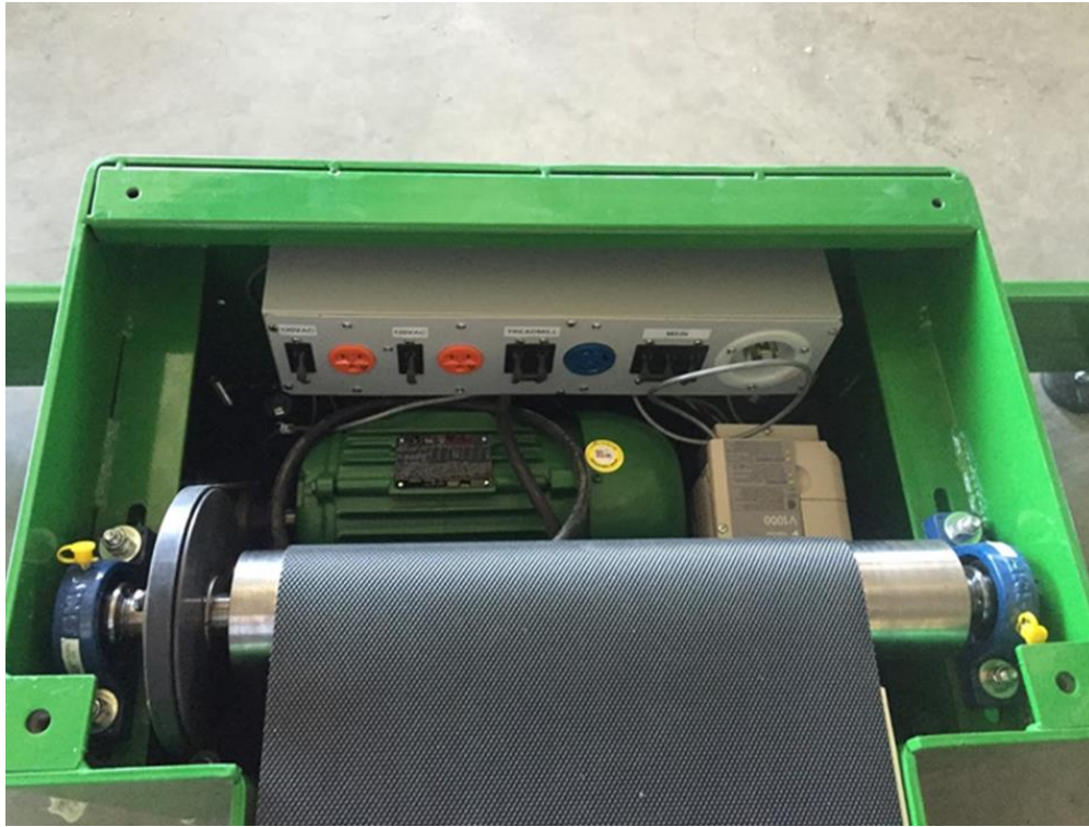
Figure 4.10: Treadmill Motor Housing Showing Motor, Electrical Panel, and VFD
