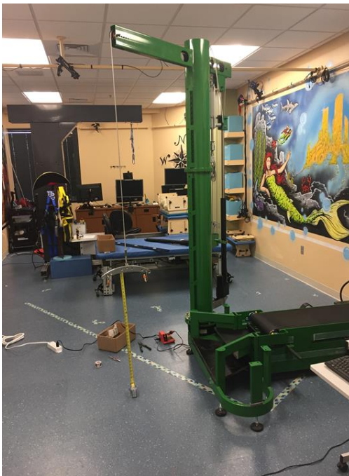
Figure 4.51: Yoke Height Low Point Dimensional Verification in Patient Pickup Location
