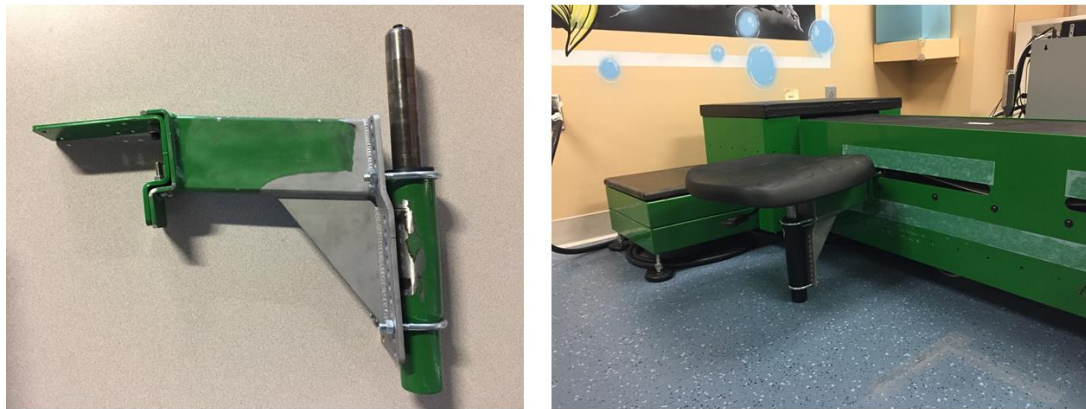
Figure 4.26: Rev. 2 Cantilever Side Seating Arm (Left) and Installed Rev. 2 Side Seating (Right)
