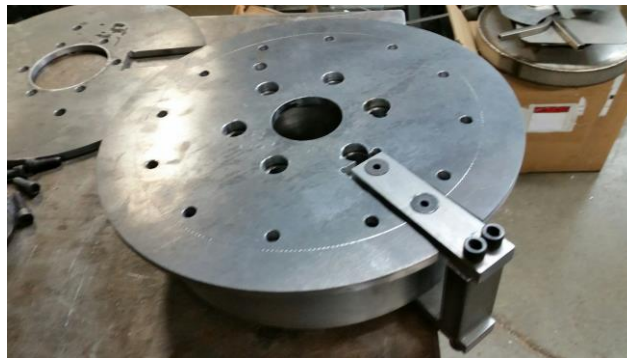
Figure 3.48: Tube Bending Die for 1"x3" Steel Tube
