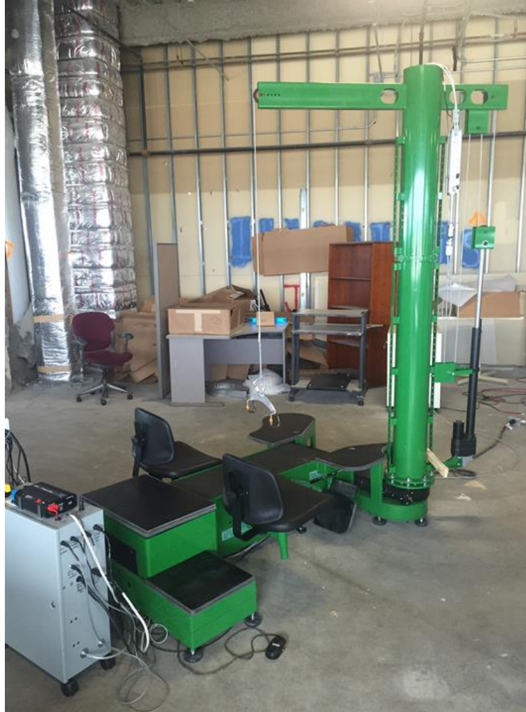
Figure 4.3: Complete BWST Assembled for Testing
