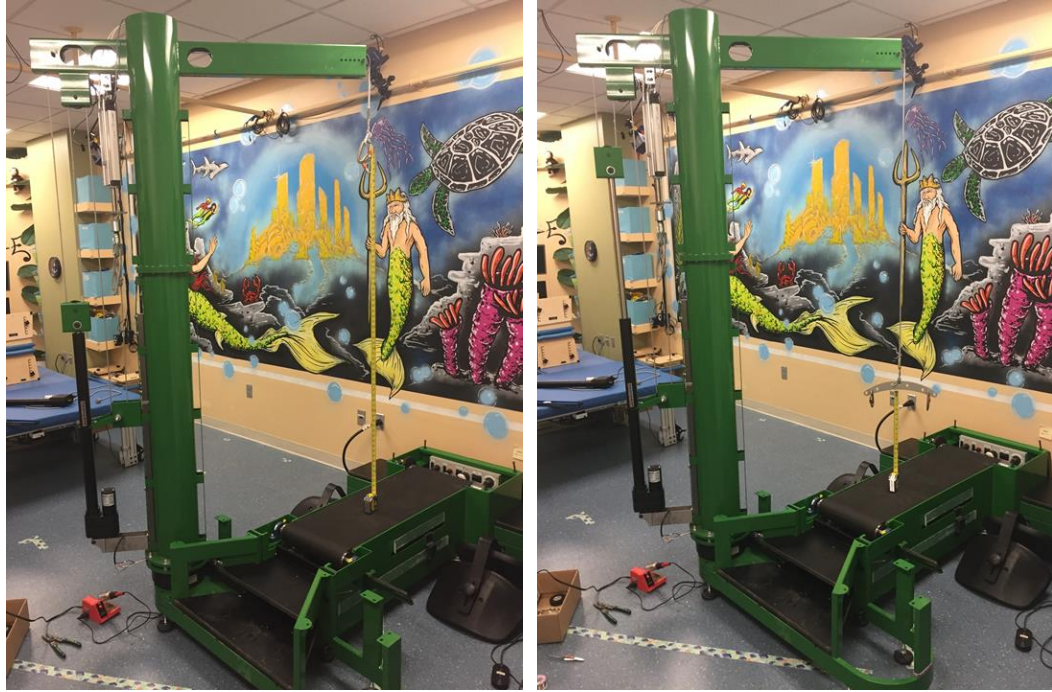
Figure 4.50: Yoke Height Dimensional Verification – High Point (Left) and Low Point (Right)
