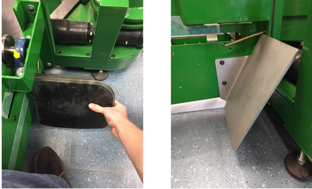
Figure 4.29: Rev. 1 Footrest Installed (Left) and Rev. 2 Footrest Installed (Right)
