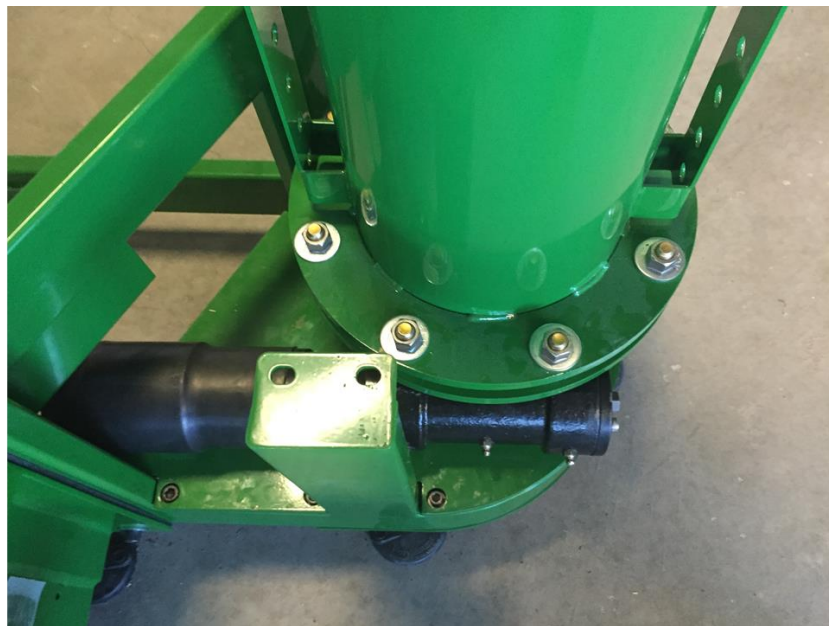
Figure 4.36: Slew Ring and Crane Attachment Point to Rear Deck
