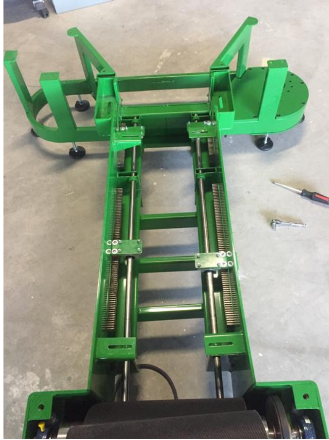
Figure 4.11: Integrated Linear Bearing and Rack System for Side Seat/Footrest within Central Treadmill
