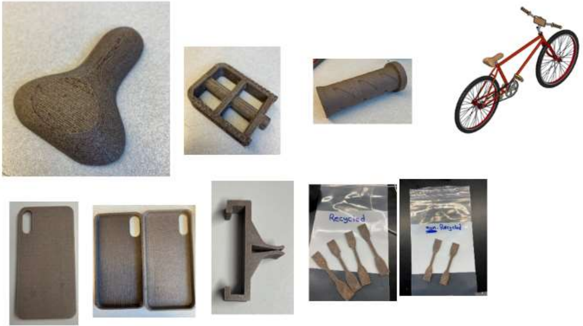
Figure 24. 3D printed bike parts with Soybean fibers filled HYTREL using FFF printers
