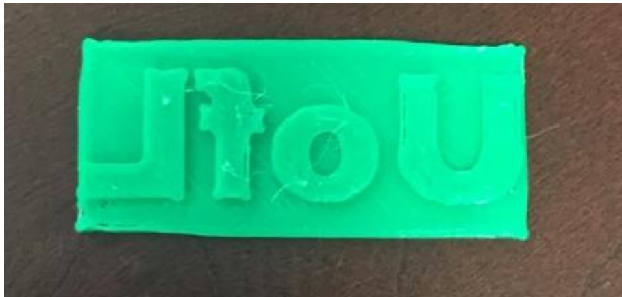
Figure 4.5 First Test Print Accidentally Mirrored Across Y-Axis
