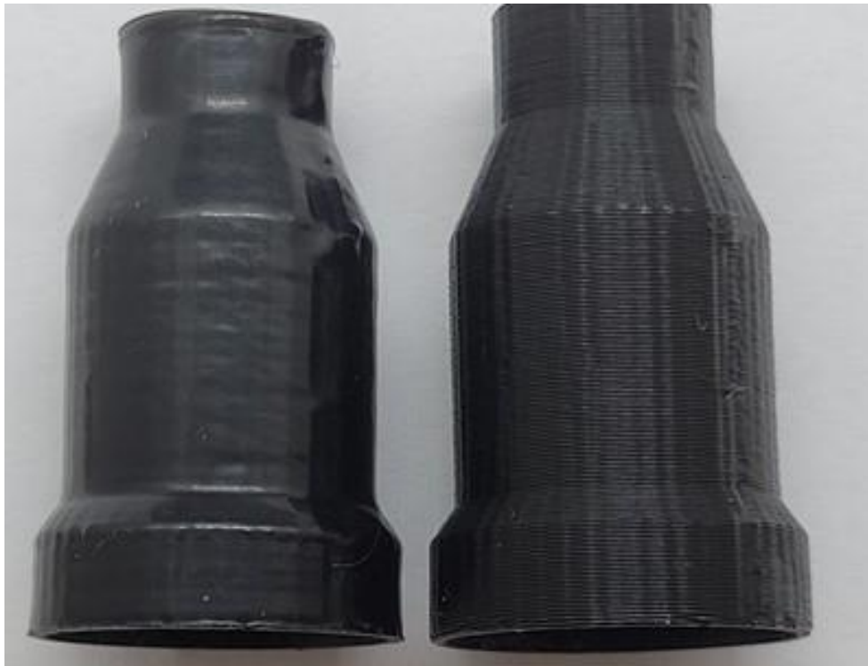
Figure 6. 9 Optical image of hose adapters printed
