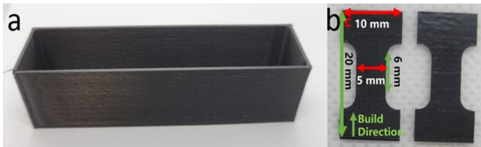
Figure 6.3 (a) Printed rectangular box without top and bottom for tensile test (b) milled tensile bars
