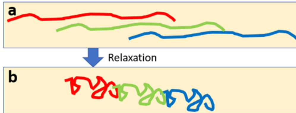
Figure 4. 8. Schematic diagram of Reptation and Relaxation(a) Initial state: stretched and disentangled; (b) After relaxation: cluster shape, entangled
