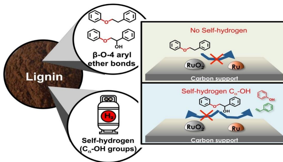
Figure 1. Graphical abstract of catalytic cleavage of the \beta -O-4 aryl ether bonds of lignin model compounds by Ru/C catalyst
